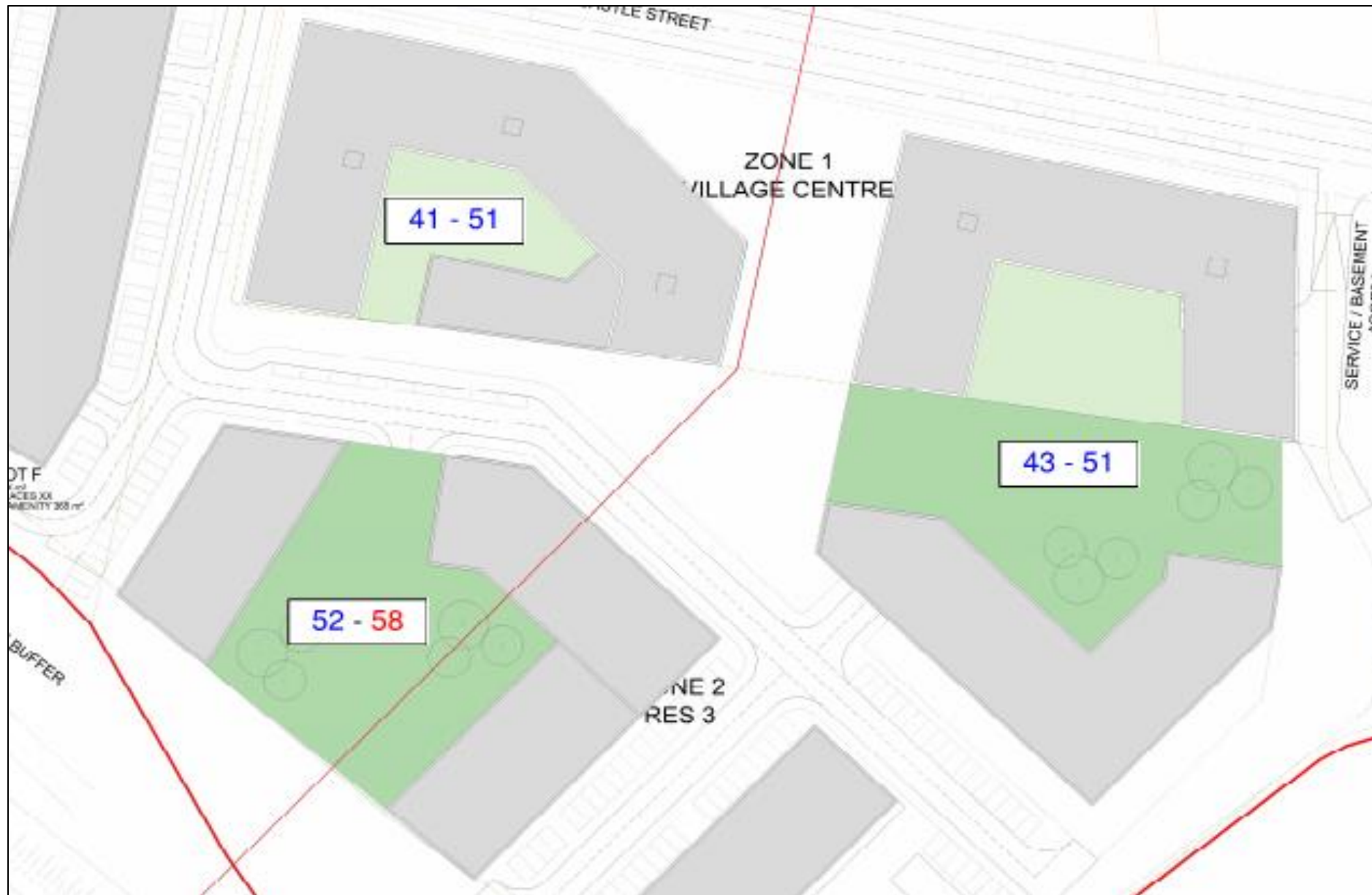
Figure A7 Predicted Ambient Noise Levels For Apartment Block Amenity Areas With 1.5m High Perimeter Wall
