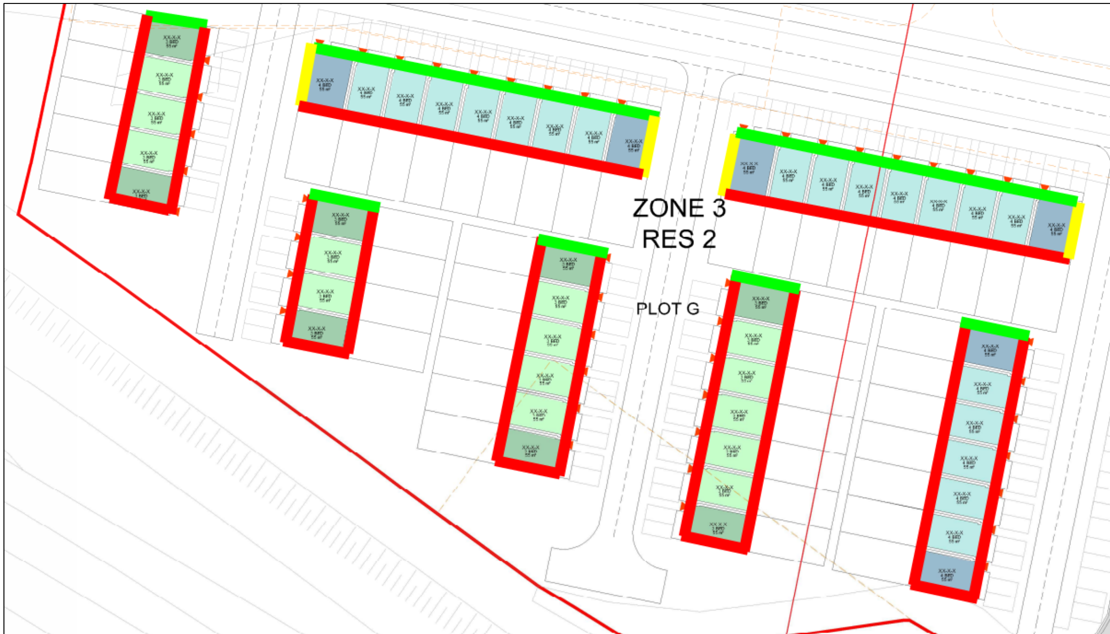
Figure A11 Dwelling First & Second Floor Glazing Sound Insulation Minimum Performance Requirements (SRI)
