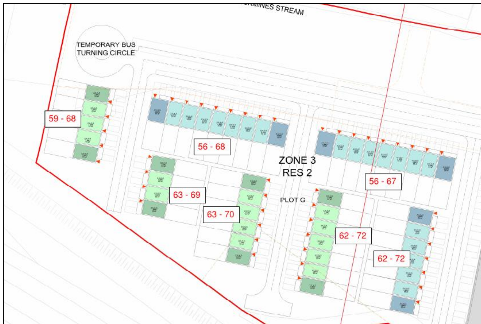
Figure A2 Predicted Ambient Noise Levels For Dwellings (No Attenuation Measures Provided)
