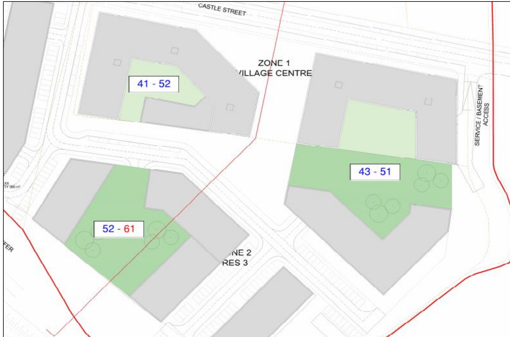
Figure A6 Predicted Ambient Noise Levels For Apartment Block Amenity Areas (No Mitigation Measures Provided)
