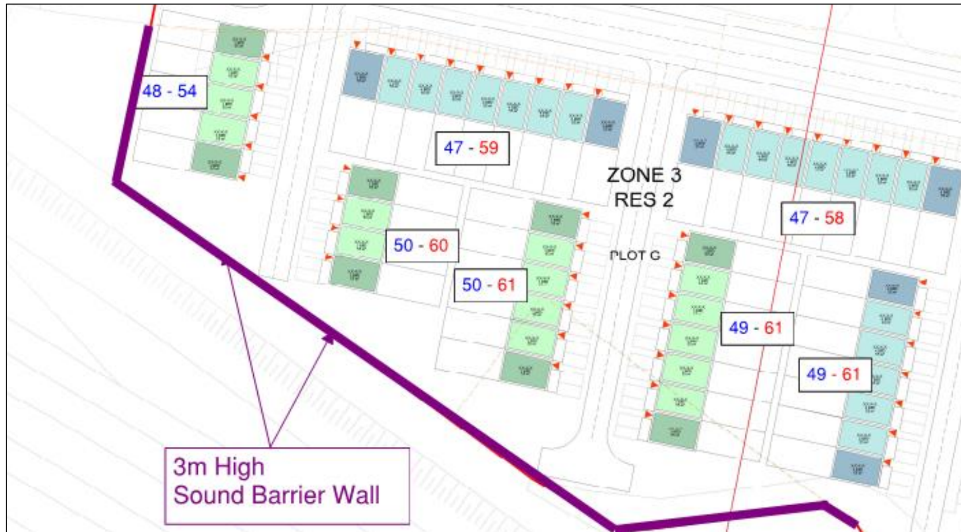
Figure A3 Predicted Ambient Noise Levels With 3m High Barrier Wall Provided Along Property Boundary
