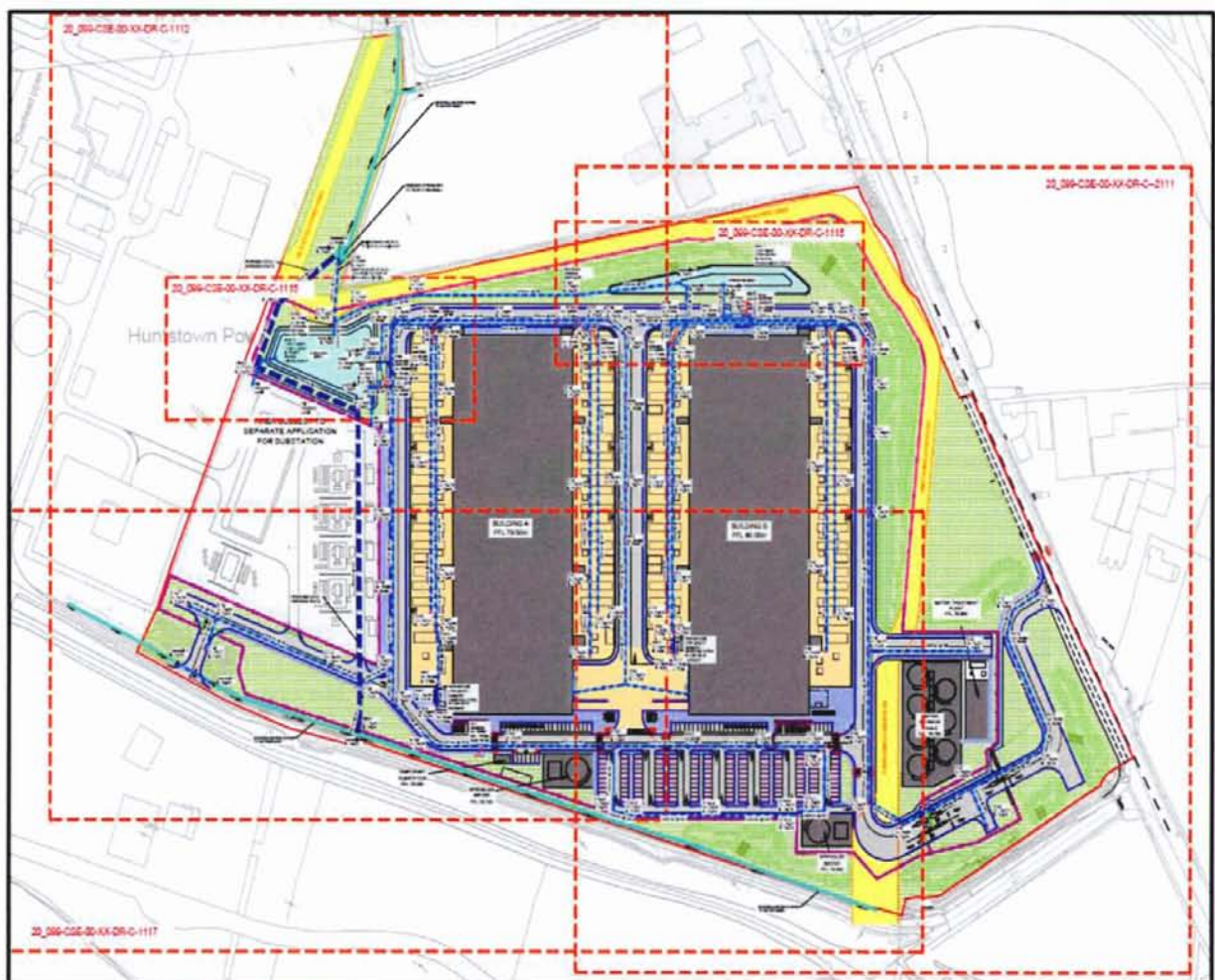
Fig 8 – Proposed Site Drainage Network
