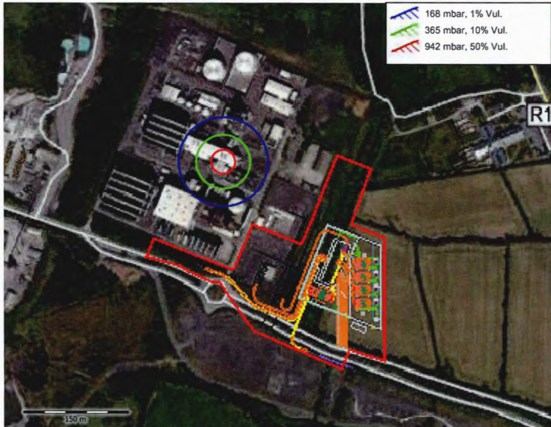
Figure 9 Natural Gas VCE in Turbine Enclosure: Outdoor Mortality Contours
