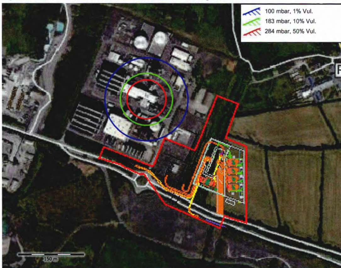
Figure 8 Natural Gas VCE in Turbine Enclosure: Blast Damage Contours
