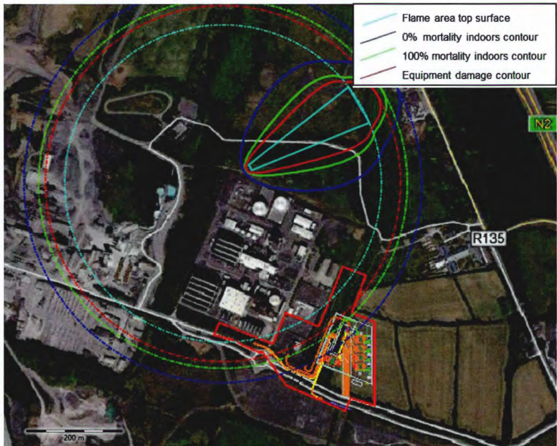
Figure 17 Natural Gas Jet Fire at GNI AGI: Indoor Mortality and Equipment Damage Contours
