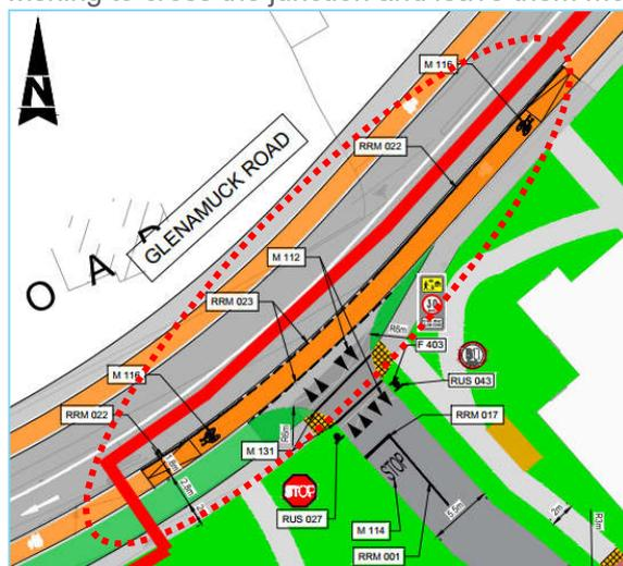
**Figure 2-12 – On road cycle track Junction 5**
