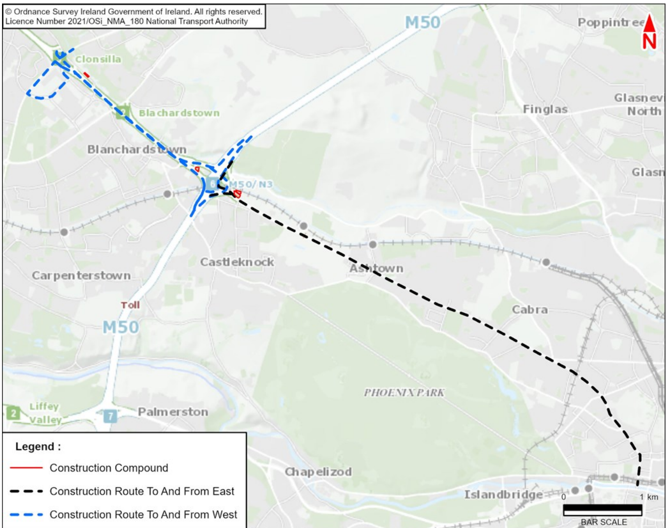
Image 5.4: Construction Vehicle Access Routes
