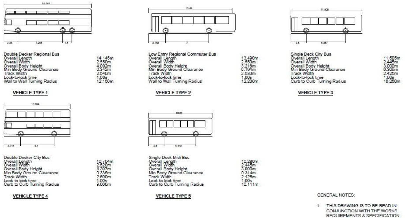
Figure 1.3 Standard Transport for Ireland Bus Specifications.
