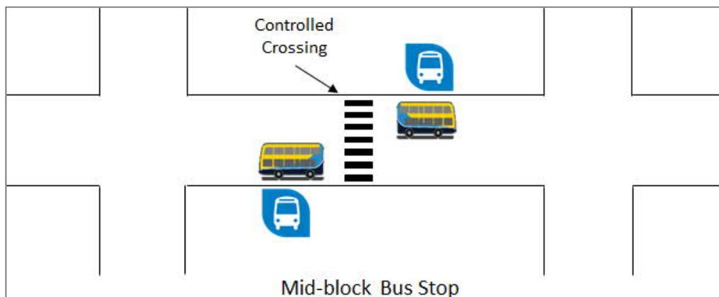
**Figure 5.10** Mid-block bus stop optimum layout.
