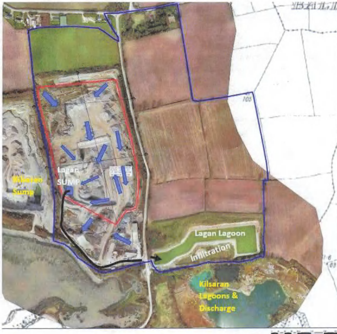
Plate 7-2 Schematic of natural runoff Surface Water Flow, Sump & Discharge to Lagoon and Infiltration area.
