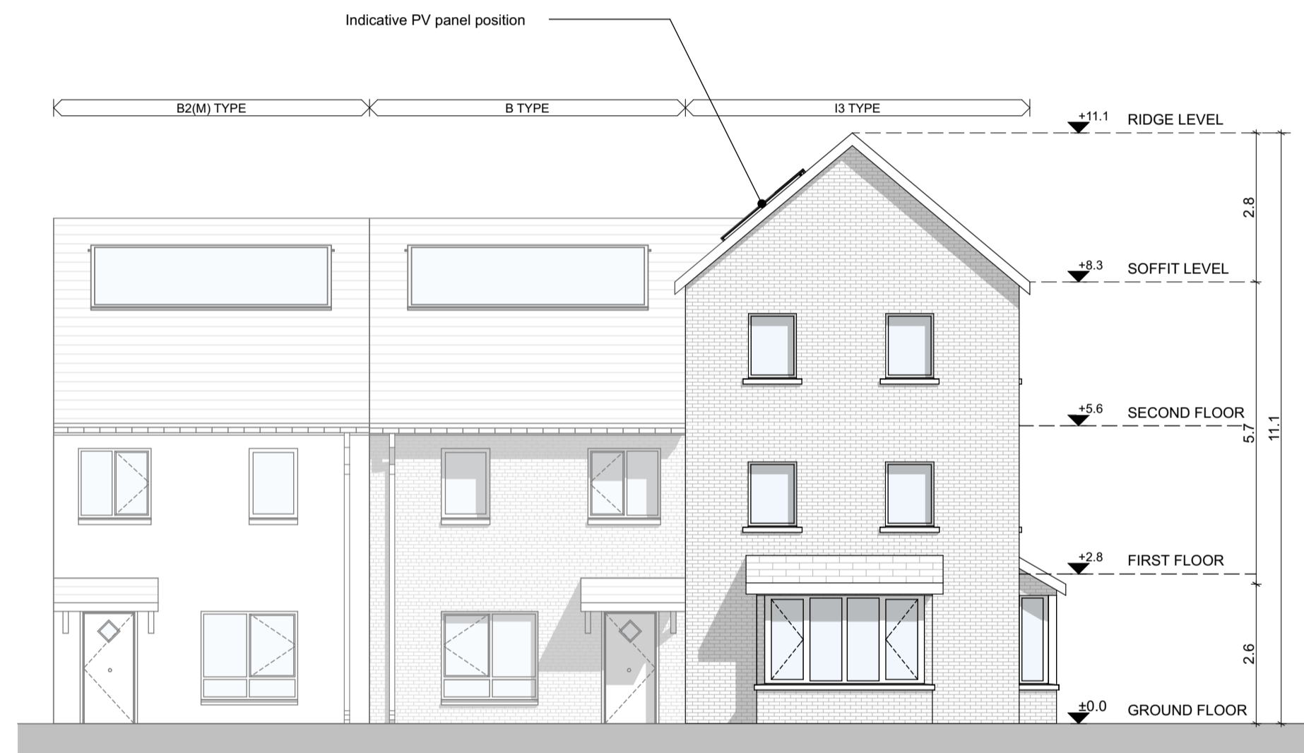
Front Elevation SCALE 1:100
