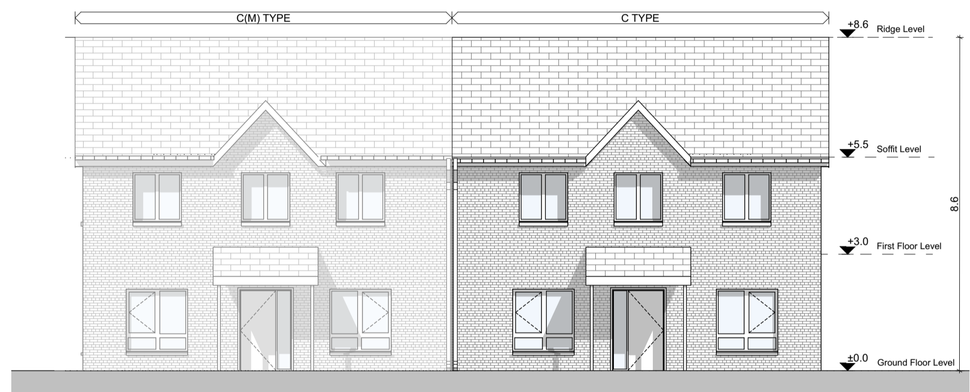
Front Elevation SCALE 1:100
