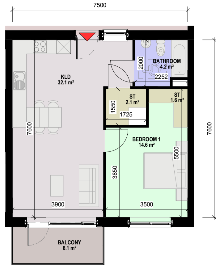
2 APT A2-6-Floor Plan -1 BED, 2 PERSON APARTMENT -NET INTERNAL AREA (NIA) Areas Shown In Plan -GROSS INTERNAL AREA (GIA) = 57m 2 1: 100
