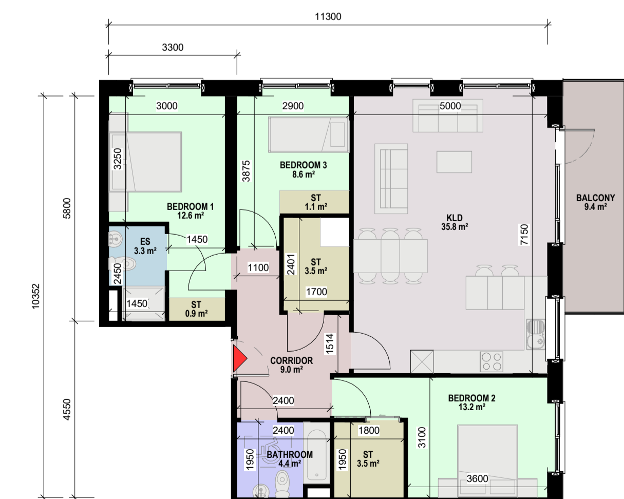
9 APT A2-3-Floor Plan -3 BED, 5 PERSON APARTMENT -NET INTERNAL AREA (NIA) Areas Shown In Plan -GROSS INTERNAL AREA (GIA) = 101.9m 2 1: 100
