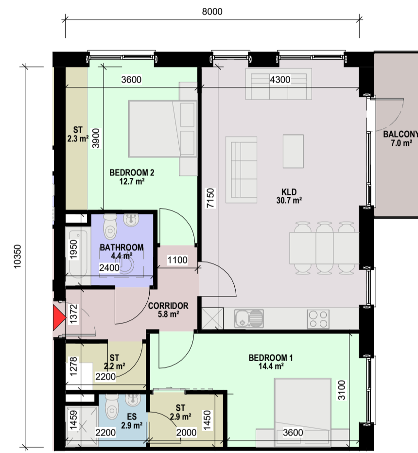
8 APT A2-8-Floor Plan -2 BED, 4 PERSON APARTMENT -NET INTERNAL AREA (NIA) Areas Shown In Plan -GROSS INTERNAL AREA (GIA) = 82.8m 2 1: 100
