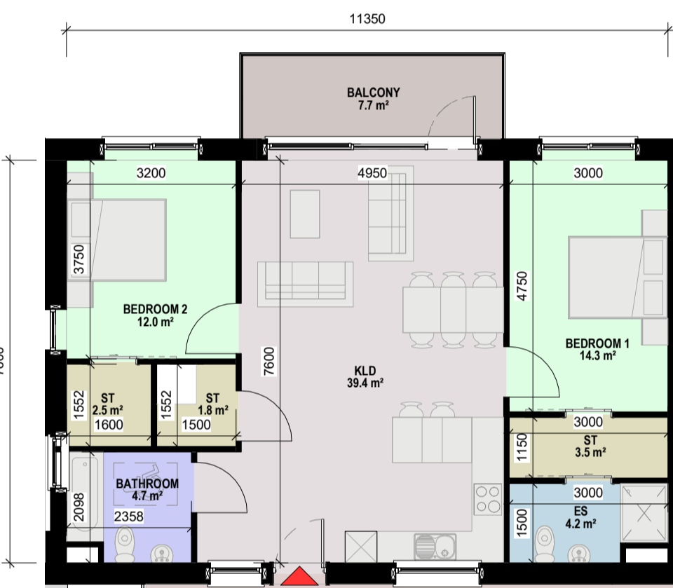
5 APT A2-2-Floor Plan -2 BED, 4 PERSON APARTMENT -NET INTERNAL AREA (NIA) Areas Shown In Plan -GROSS INTERNAL AREA (GIA) = 86.3m 2 1: 100
