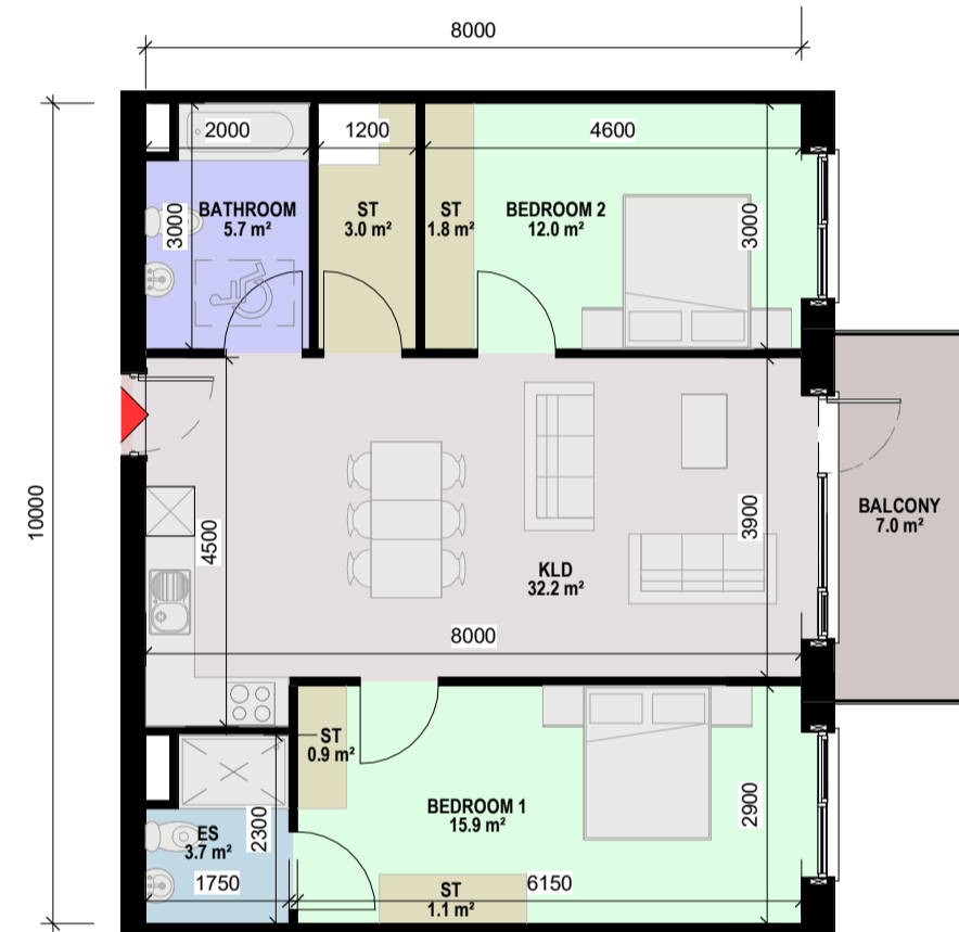
6 APT A2-5-Floor Plan -2 BED, 4 PERSON APARTMENT -NET INTERNAL AREA (NIA) Areas Shown In Plan -GROSS INTERNAL AREA (GIA) = 80.00m 2 1: 100
