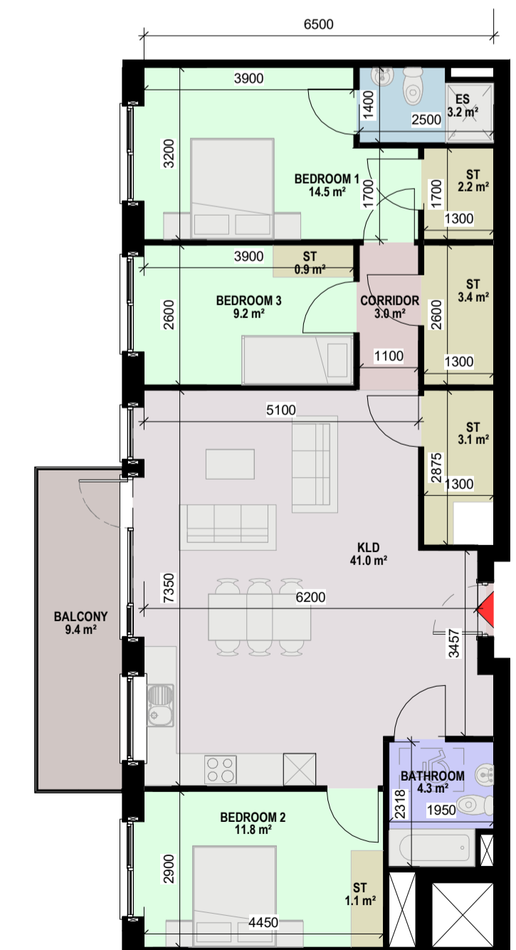
11 APT A2-4-Floor Plan -3 BED, 5 PERSON APARTMENT -NET INTERNAL AREA (NIA) Areas Shown In Plan -GROSS INTERNAL AREA (GIA) = 102.5m 2 1: 100
