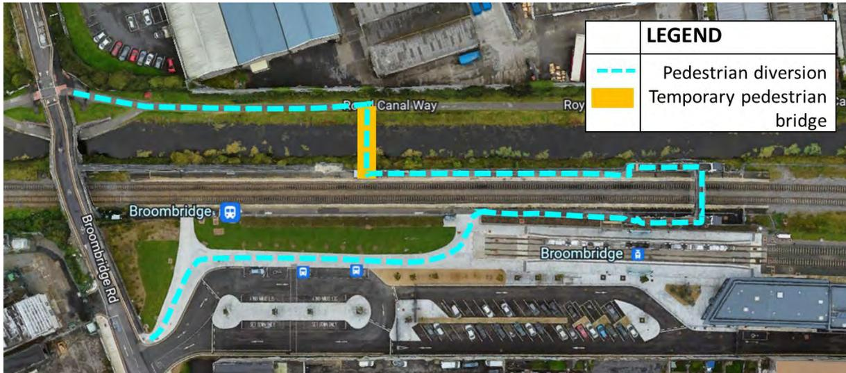
Figure 5-233 Pedestrian diversion via temporary ramp at OBG5
