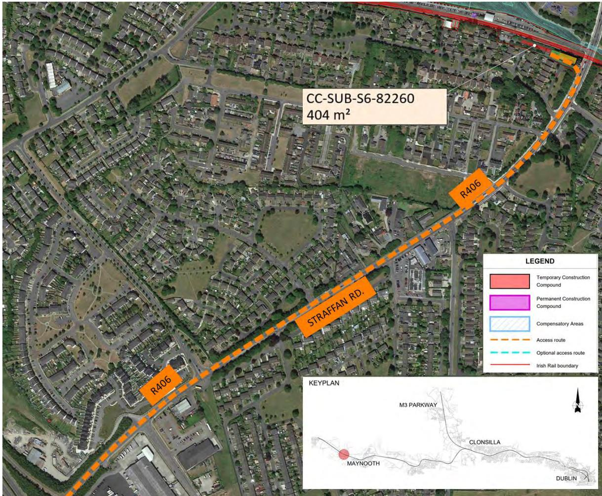
**Figure 5-332 Maynooth substation compound and haulage route**
