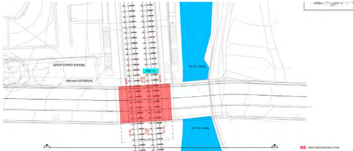
**Figure 5-306 Plan of OBG14 deck reconstruction**
