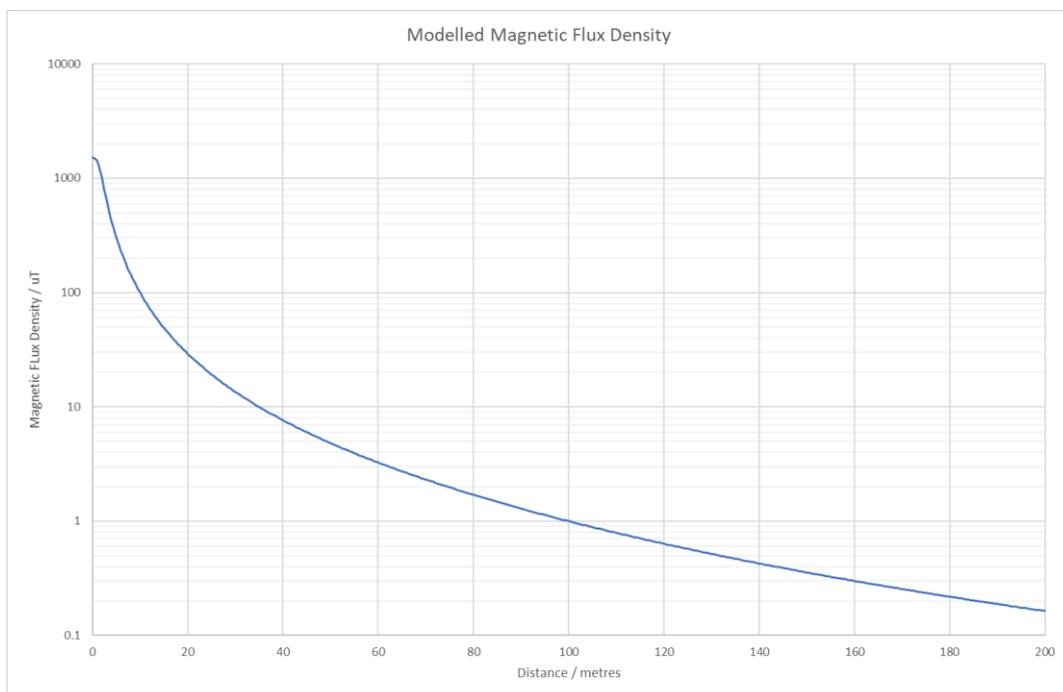
**Figure 22-6 Modelled DC Magnetic flux density for worst-case conditions**
