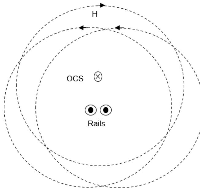
**Figure 22-4 DC magnetic field around rails and OCS**
