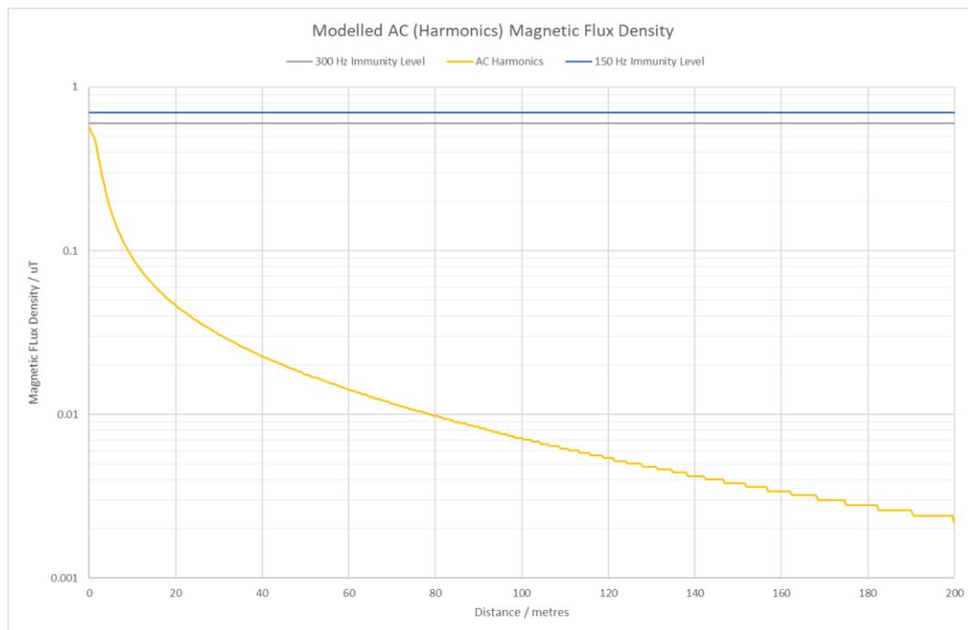
**Figure 22-8 Modelled magnetic flux density of harmonics for worst-case conditions**
