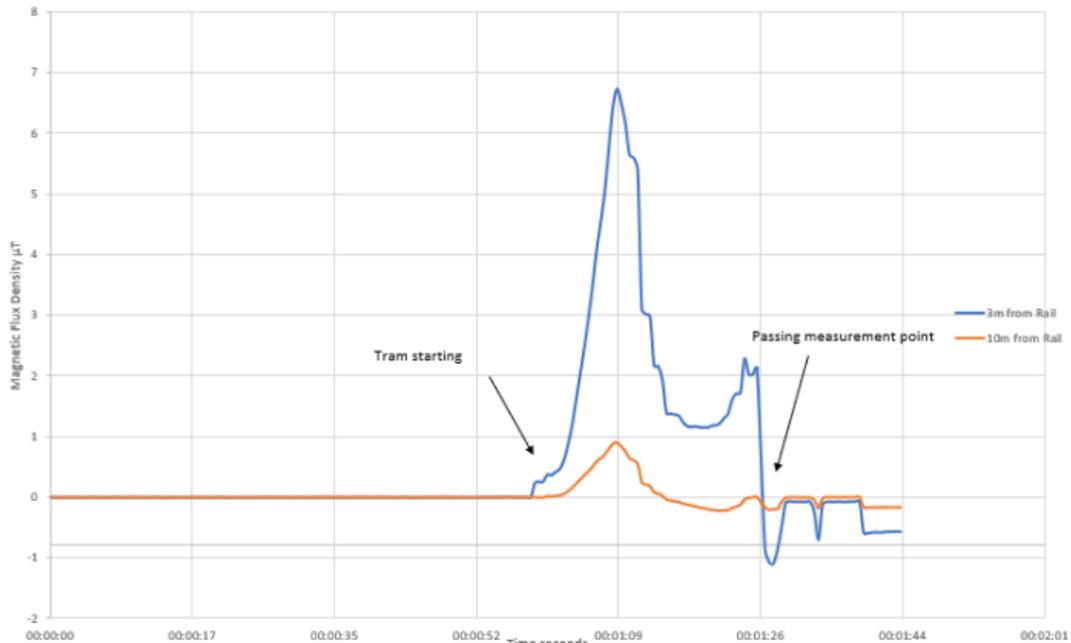
**Figure 22-5 Magnetic flux density electrified train passing measuring point at 3 m and 10 m distance**
