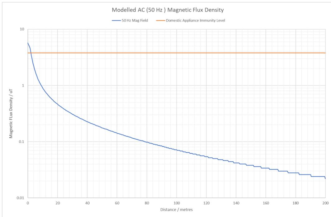
**Figure 22-7 Modelled 50 Hz Magnetic flux density for worst-case conditions**
