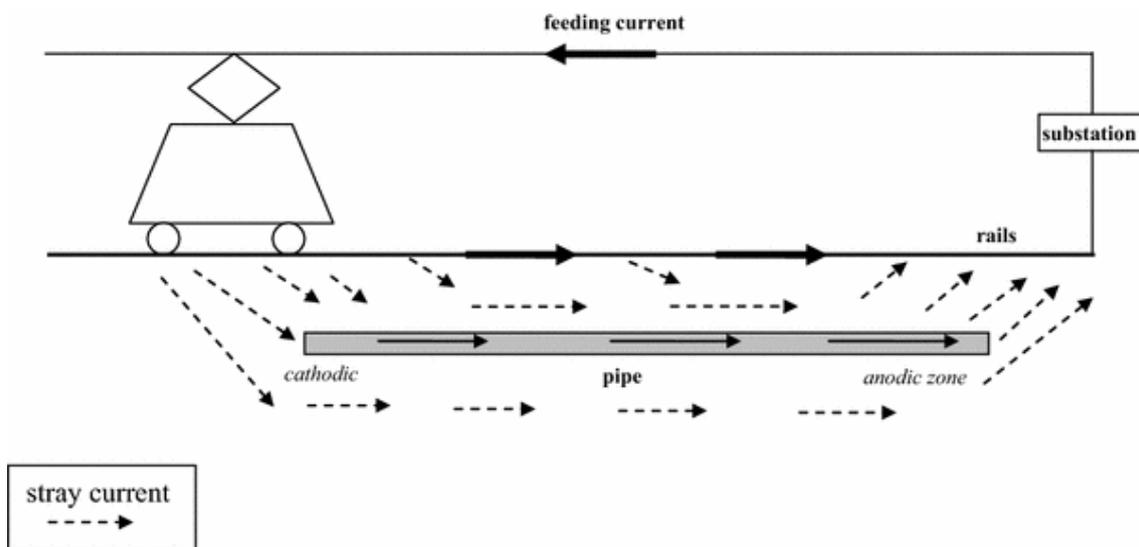
**Figure 22-9 Illustration of stray currents from an electrified rail system**
