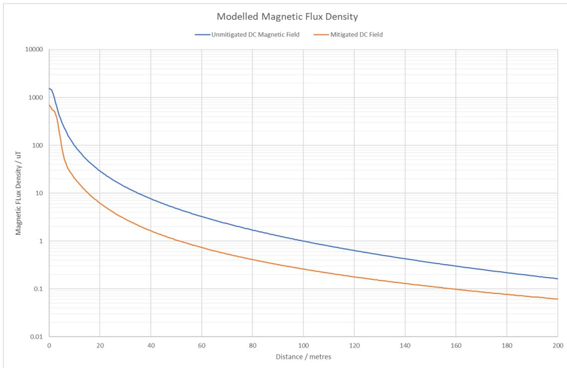
**Figure 22-12 Unmitigated Vs mitigated DC Magnetic Field profile**
