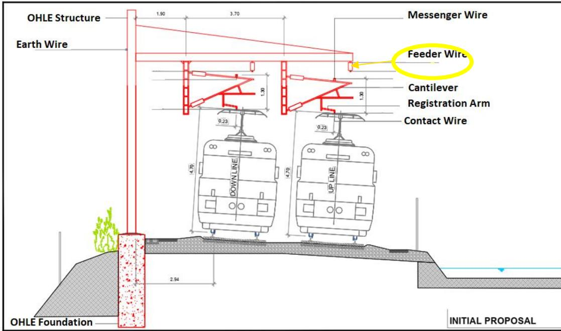
**Figure 22-10 Standard OHLE layout**
