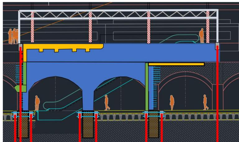
Figure 45. Sketch showing the structural solution for a void containing an escalator
