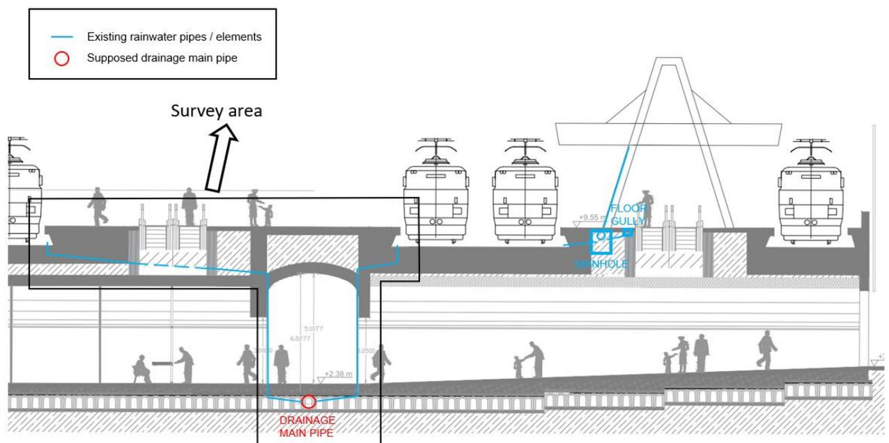
Figure 68 – Rainwater drainage system. Supposed current solution
