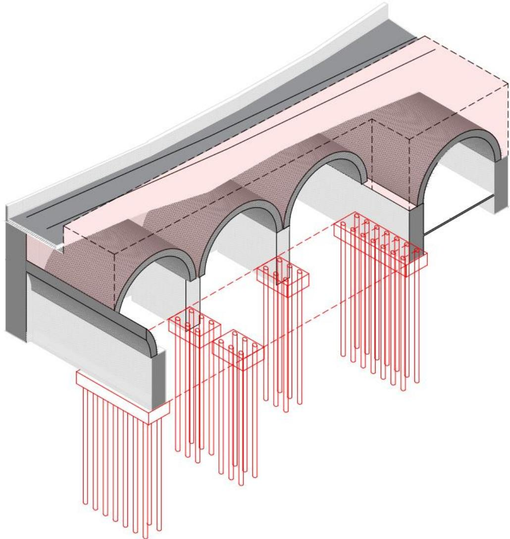
Figure 50. Axonometric view step 1, foundations.
