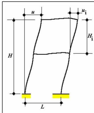
**Figure 40 - Definition of Horizontal displacements. Source: I.S. EN-1990-2002+A1-2005, A.1.4.3**
