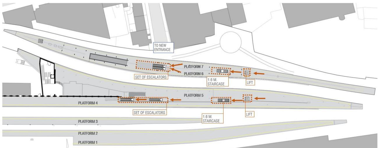
**Figure 17. Platform facilities. Proposed additional means of access to the platforms**
