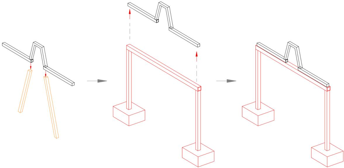
**Figure 53. Cut of the existing structure. New steel structure and foundations on platform.**
