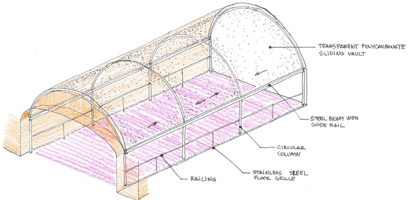
**Figure 34. Sketch of the transparent polycarbonate umbrella inside the vault**
