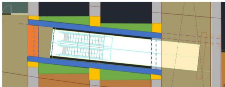
Figure 44. Sketch of a plan view of the new void
