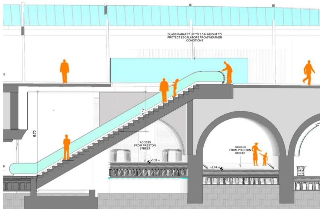
Figure 49. Section of the analysed escalator and opening
