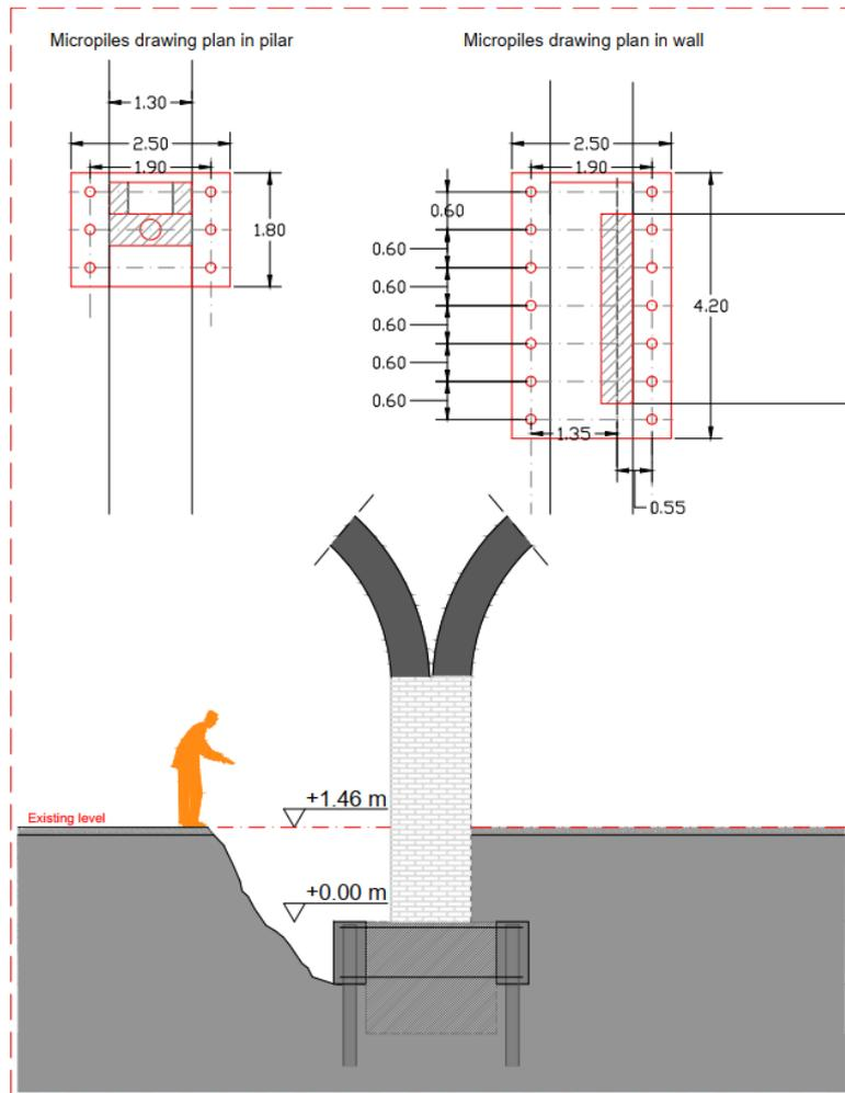
Figure 51. Elevation drawing of excavation up to base of pile cap. Plan drawing of two types of foundations.
