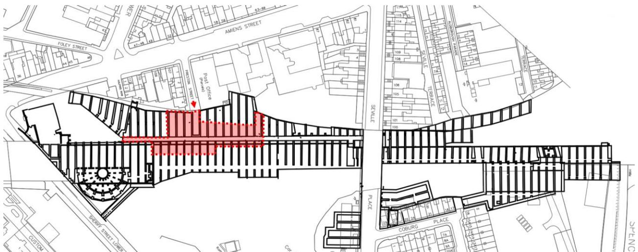
**Figure 21. Vaults area to be refurbished. The new entrance to the station is located at Preston St.**
