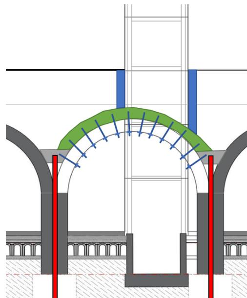
Figure 47. Sketch showing the structural solution for a void containing a lift
