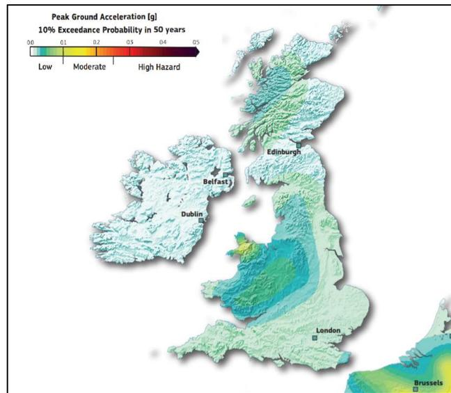
Figure 38 – Peak ground acceleration [g] 10% exceedance probability in 50 years. (Source: SHARE European Seismic Hazard Map for Peak Ground Acceleration, 10% Exceedance in 50 years)
