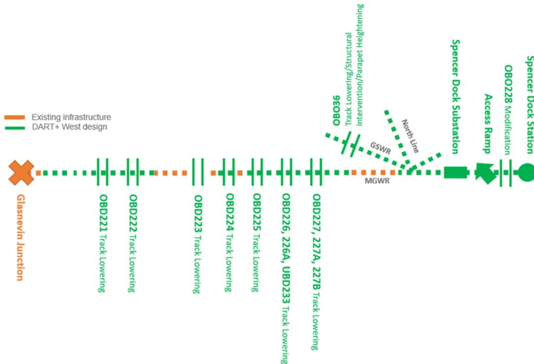
**Figure 4-8 Scheme of the DART+ West interventions in Zone B**
