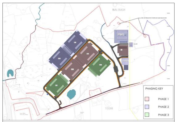
*Figure 2.2* Intended Construction Phasing for the proposed Masterplan (ART-ARC-SP-00-DR-A-0003).
