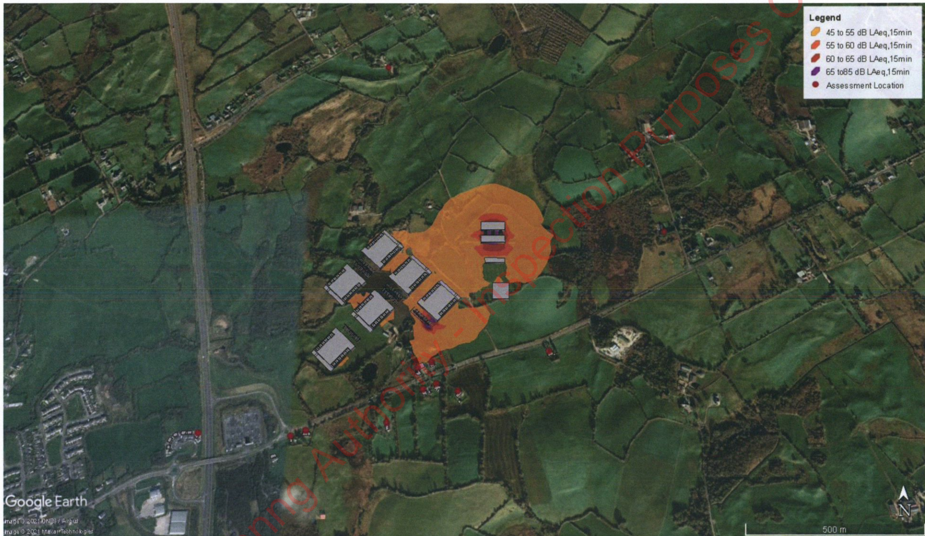
Figure 9.8 Scenario C Proposed Data Storage Facility (current planning application) – Generator Testing Noise Contour (Extent of 45dB(A) noise contour)
