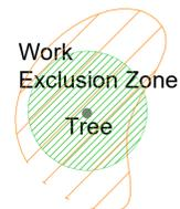
Protective fence line to protect work exclusion zone around trees being retained.
