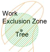
Protective fence line to protect work exclusion zone around trees being retained.
