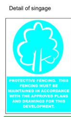
The tree protection fencing is to be erected enclosing the root protection areas around the trees being retained as shown on this drawing and appendix 1. In some areas, the site hoarding may be sufficient to act as the protective fencing if the tree and its root zone are positioned outside and no works are envisaged within the area outside the site hoarding. This will need to be discussed and agreed at the initial site meeting.
