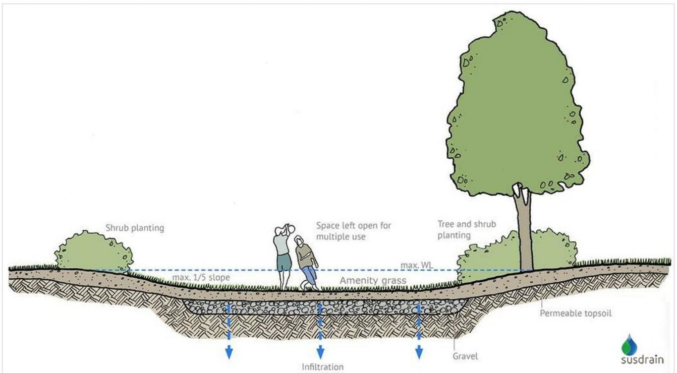
Diagram 4.10: Typical Infiltration Basin (Taken from Susdrain)
