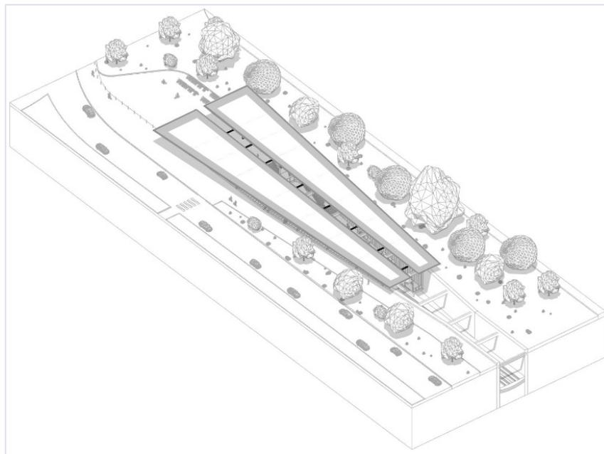
**Diagram 4.3: Typical Footprint of a Station in Retained Cut**
