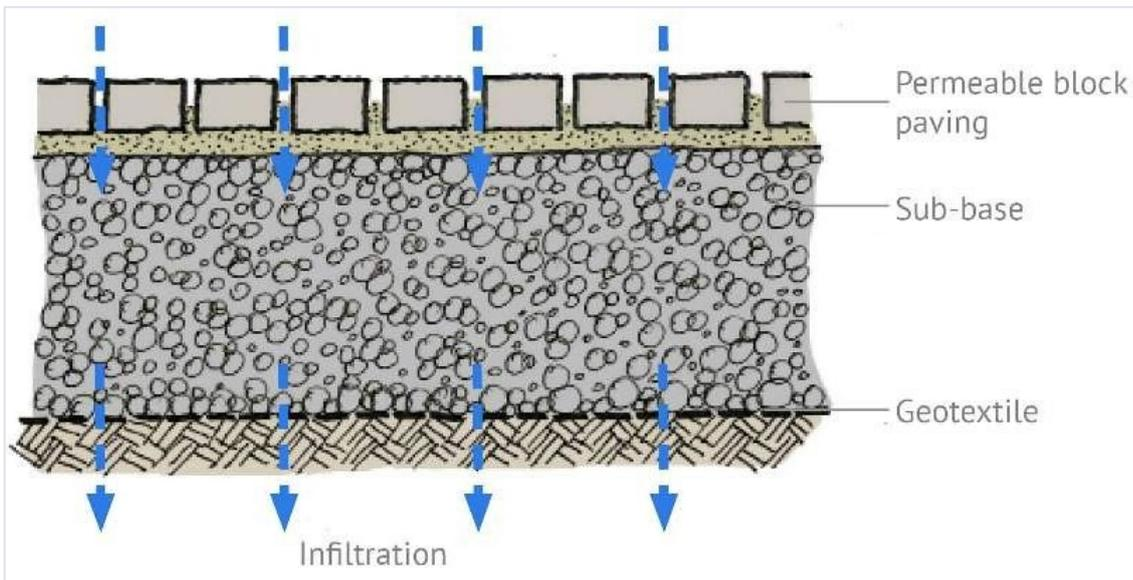
Diagram 4.11: Typical Pervious/Permeable Pavement (Taken from Susdrain)
