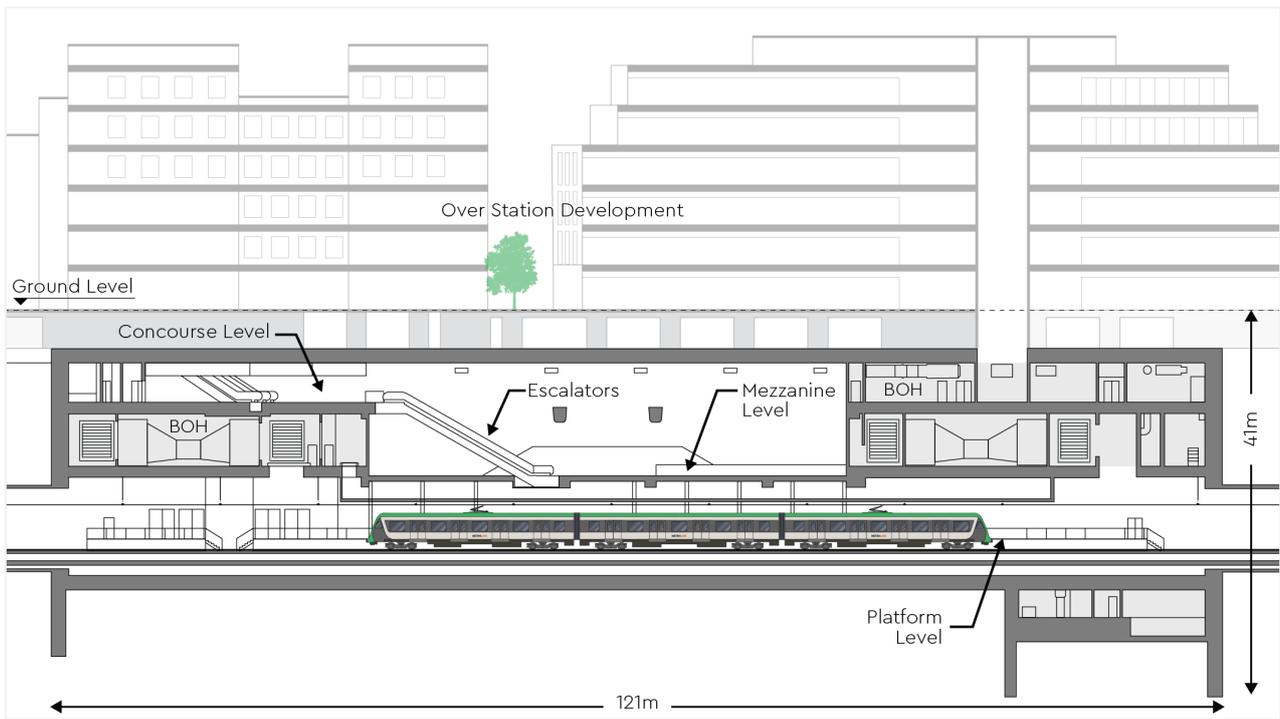
Diagram 4.89: Longitudinal Cross Section of O'Connell Street Station
