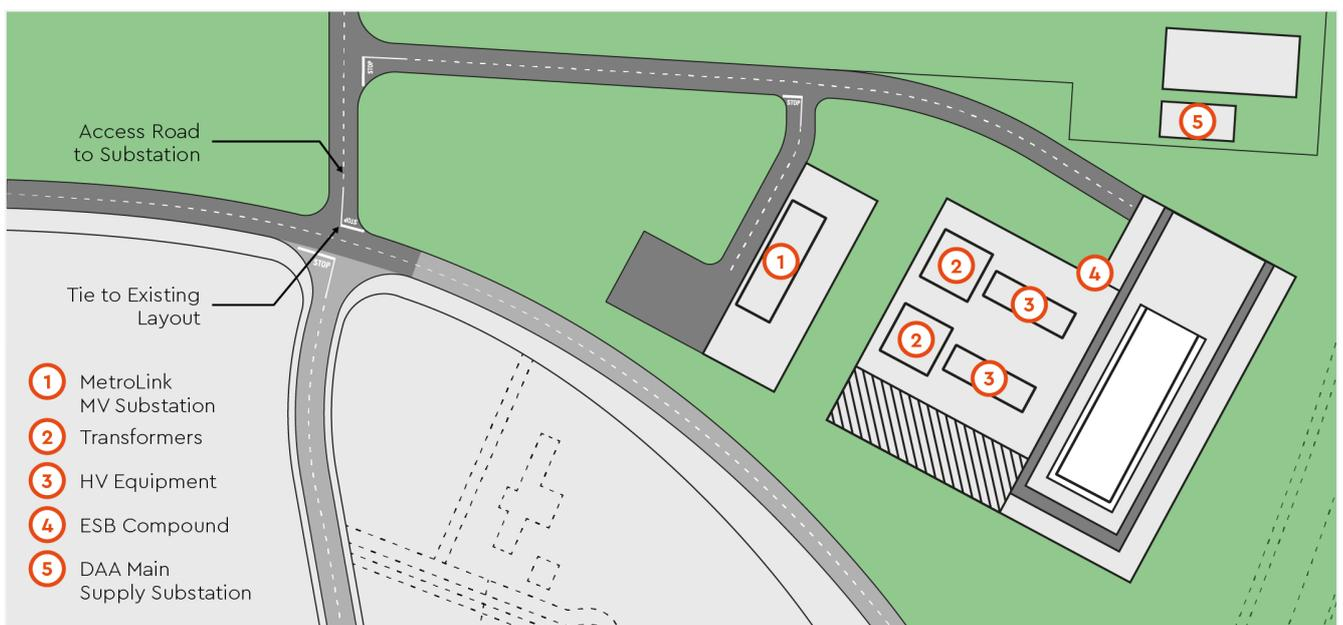
**Diagram 4.57: Layout of the Transmission Substation near DANP**
