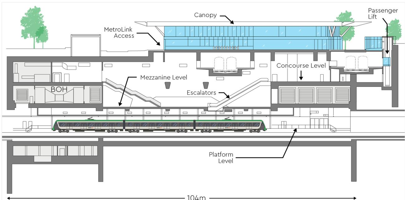
**Diagram 4.84: Longitudinal Cross Section of Glasnevin Station**
