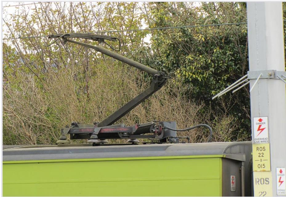
**Diagram 4.27: Example of a Pantograph above a Train**
