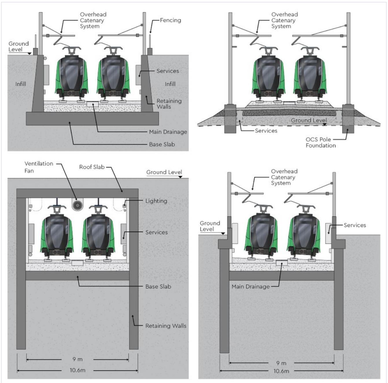
Diagram 4.20: Surface and Cut Sections to be used along the Alignment (Clockwise from Top Right, Surface, Retained Cut, Cut and Cover, and U-cut)
