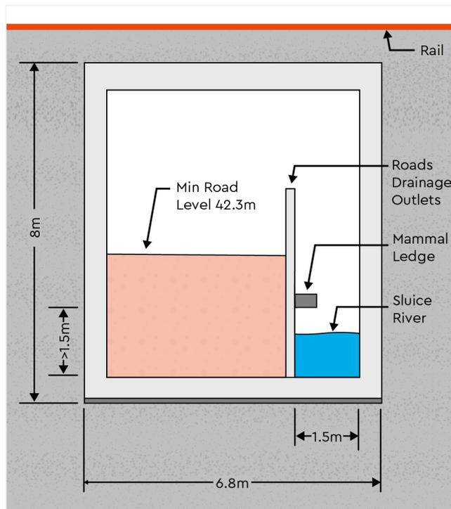
**Diagram 4.52: Sluice River Culvert Cross-Section Including Road Underpass at Ch 5+762**
