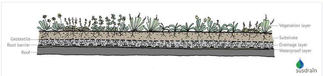
**Diagram 4.8: Typical Green Roofs (Taken from Susdrain)**
