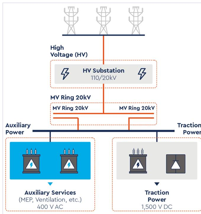
**Diagram 4.25: Schematic of MetroLink's Operational Power Supply**
