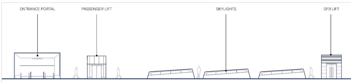
**Diagram 4.6: Sketches of Common Components at Ground Level**
