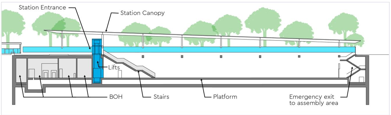
**Diagram 4.14: General Long Section Arrangement of a Retained Cut Station**
