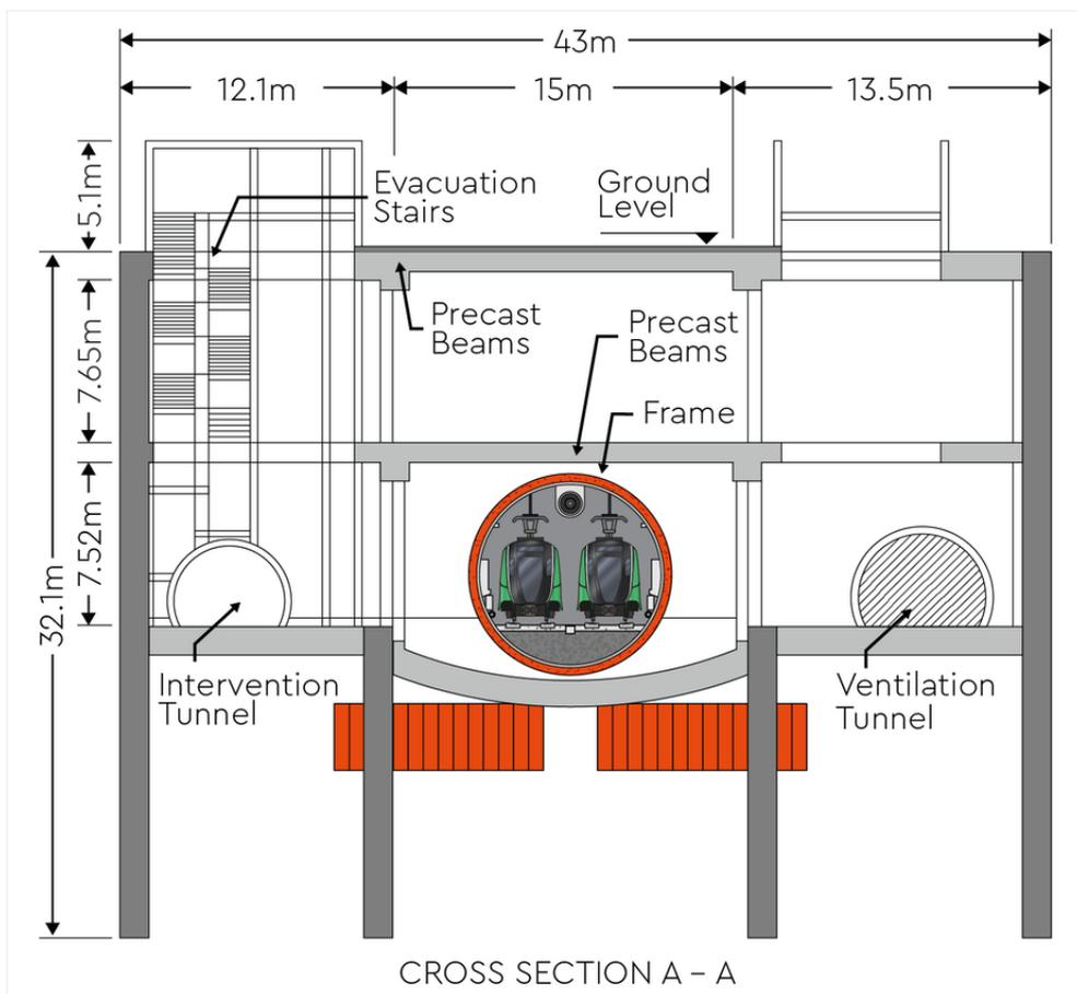
Diagram 4.61: Cross Section of DASP Showing the Evacuation and Ventilation Tunnels
