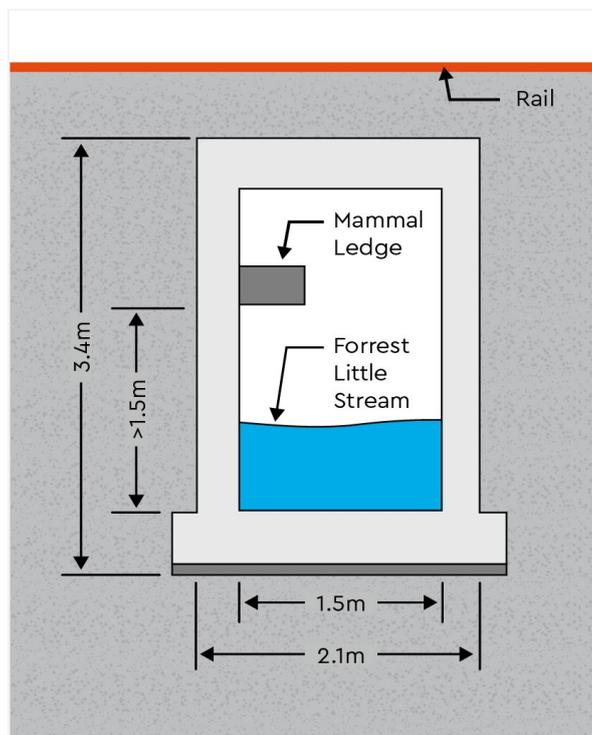
**Diagram 4.53: Forrest Little Stream Culvert Cross-Section at Ch 5+963**
