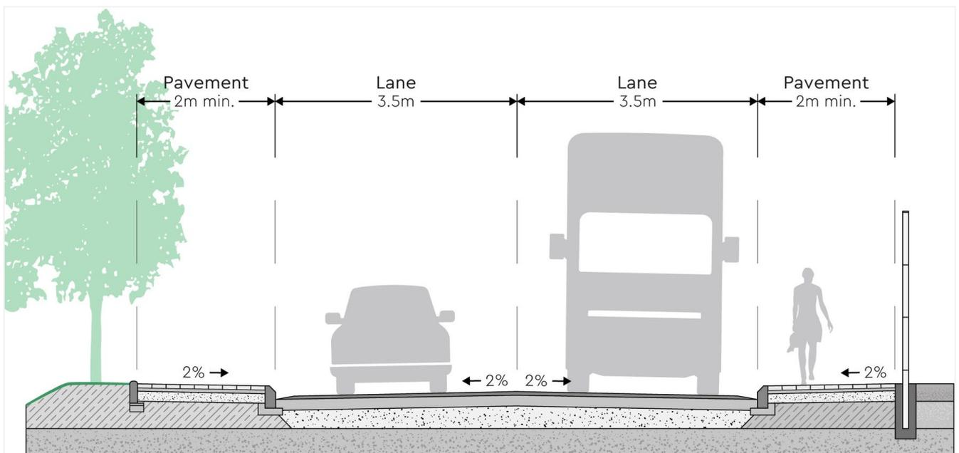
**Diagram 4.66: Typical Cross Section of the Depot Access Road**
