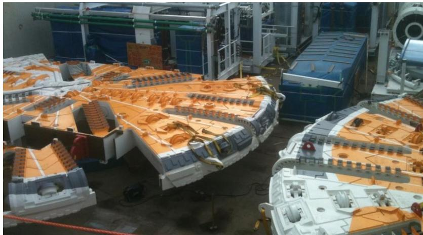
**Diagram 4.10: Three-piece Cutterhead in a Barge**
