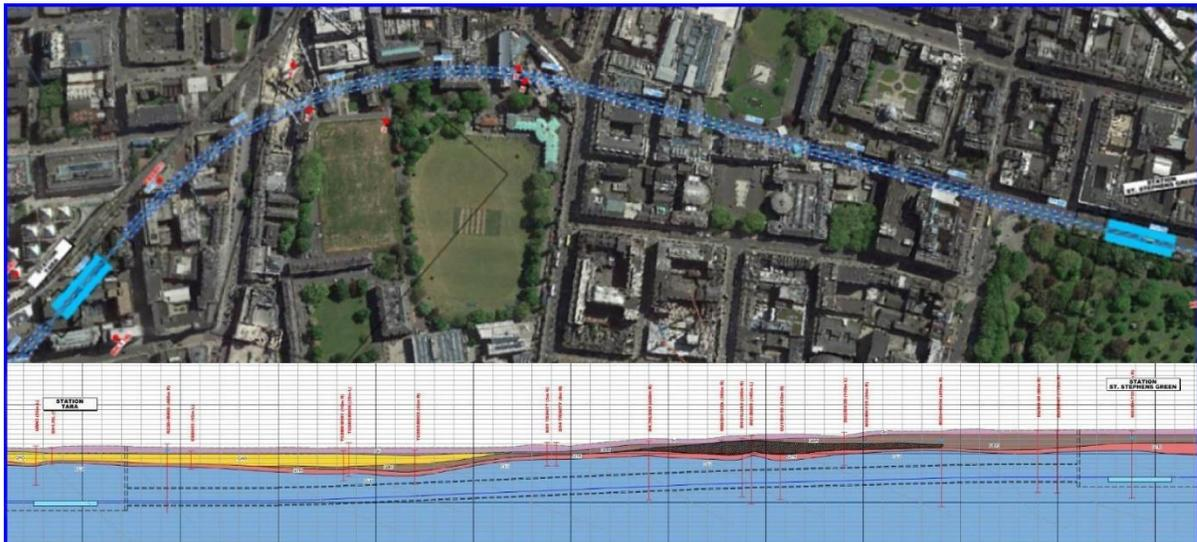
Diagram 3.13: Geologic Profile for TBM Drive C8- Tara Station to St Stephen's Green
