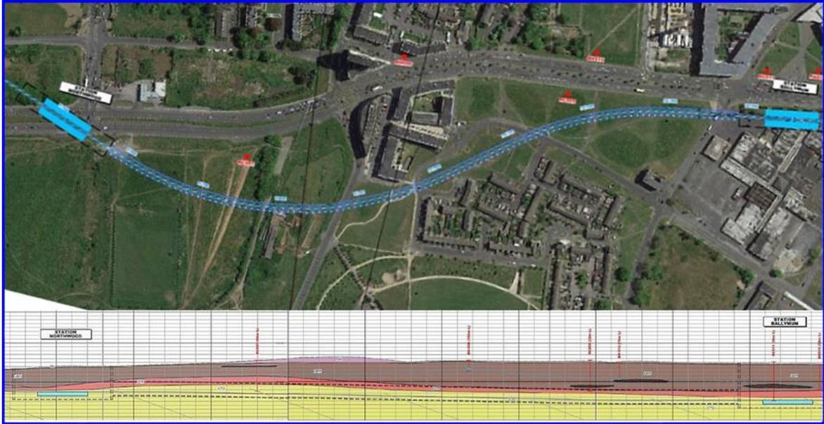
**Diagram 3.6: Geologic Profile for TBM Drive C1: Northwood to Ballymun**
