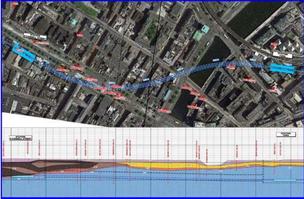
**Diagram 3.12: Geologic Profile for TBM Drive C7- O'Connell Street to Tara**
