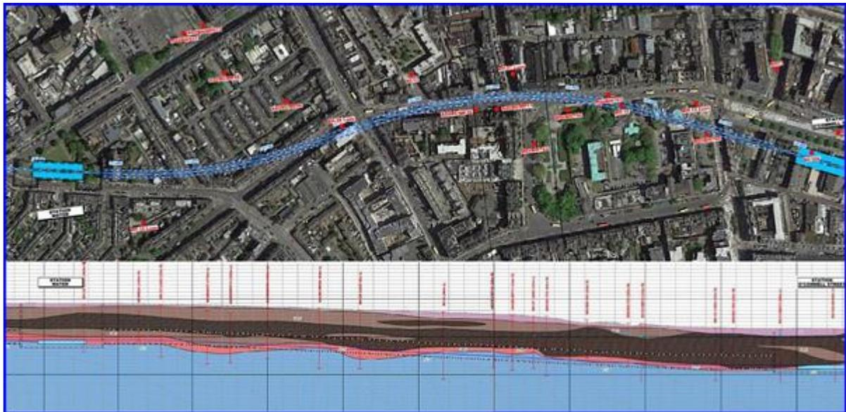
Diagram 3.11: Geologic Profile for TBM Drive C6- Mater to O'Connell Street
