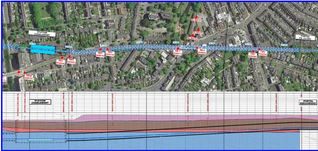
Diagram 3.15: Geologic profile for TBM drive C10- Charlemont to south of Charlemont TBM Burial Site
