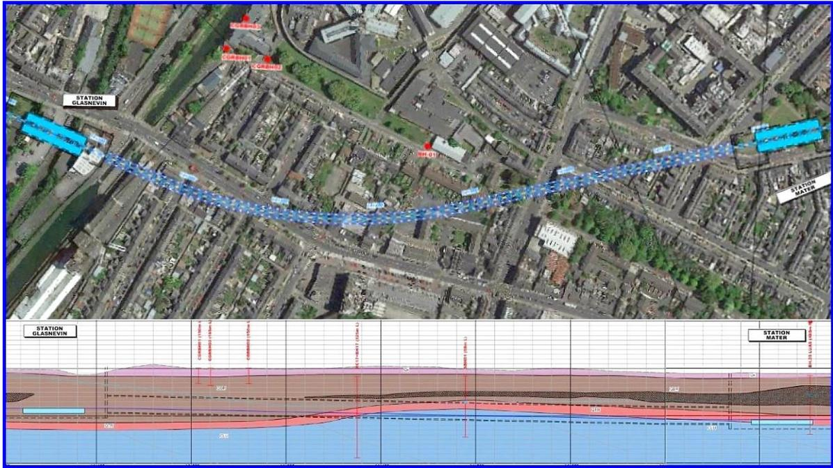
**Diagram 3.10: Geologic profile for TBM drive C5- Glasnevin to Mater**
