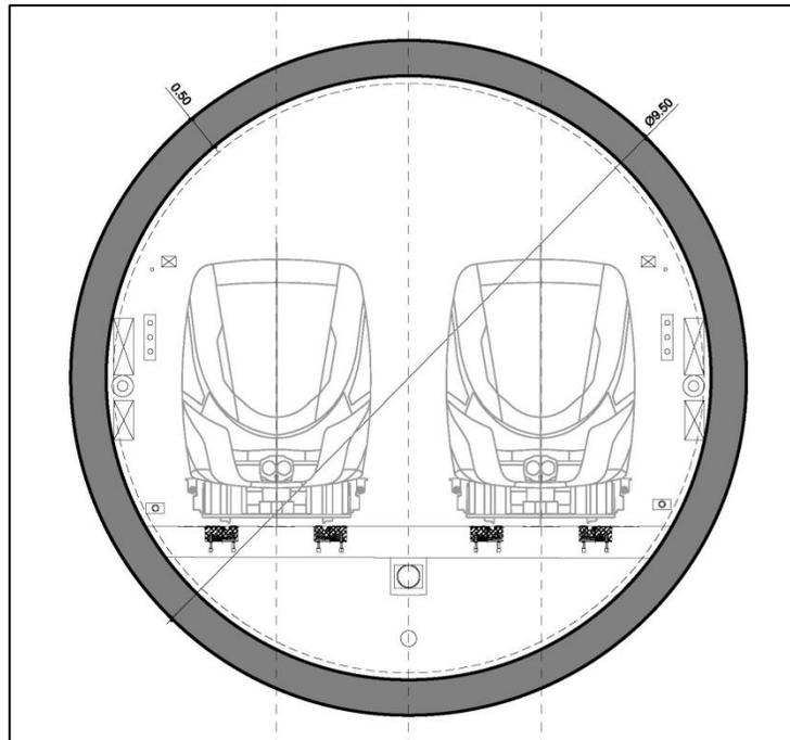
**Diagram 4.1: The tunnel cross-section is shown with an internal diameter of 8.5m, and an external diameter of 9.5m**
