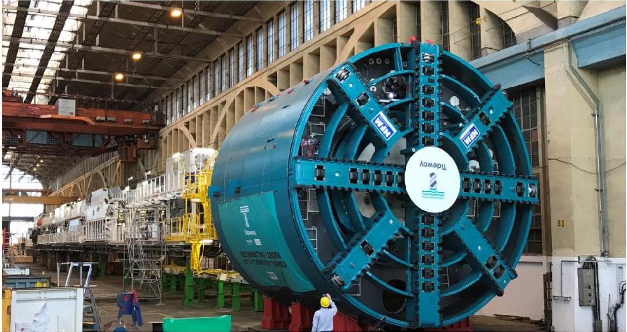
**Diagram 4.19: TBM and gantries in factory ready for Factory Acceptance Tests**
