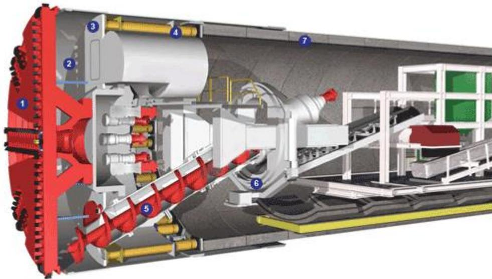
**Diagram 4.2: Schematic of a typical EPB machine (from Herrenknecht)**
