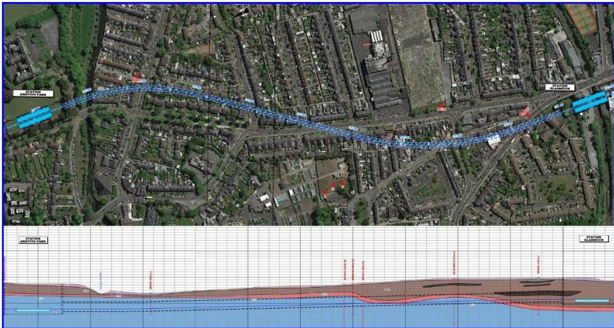
Diagram 3.9: Geologic Profile for TBM Drive C4- Griffith Park to Glasnevin
