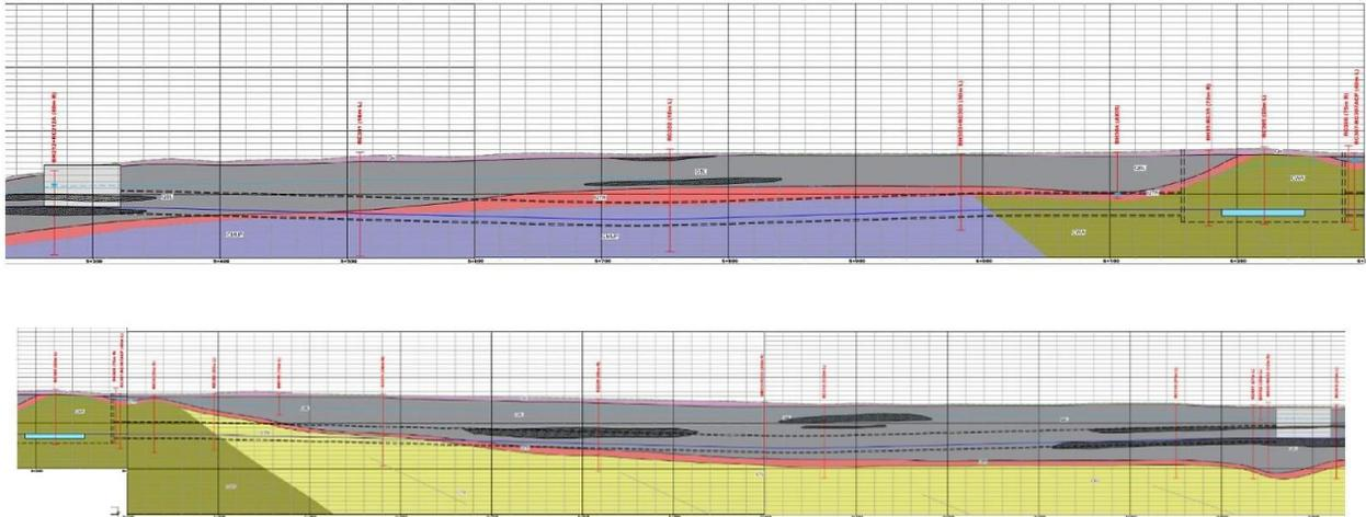
**Diagram 3.4: Geologic Profile for the Dublin Airport Tunnel**
