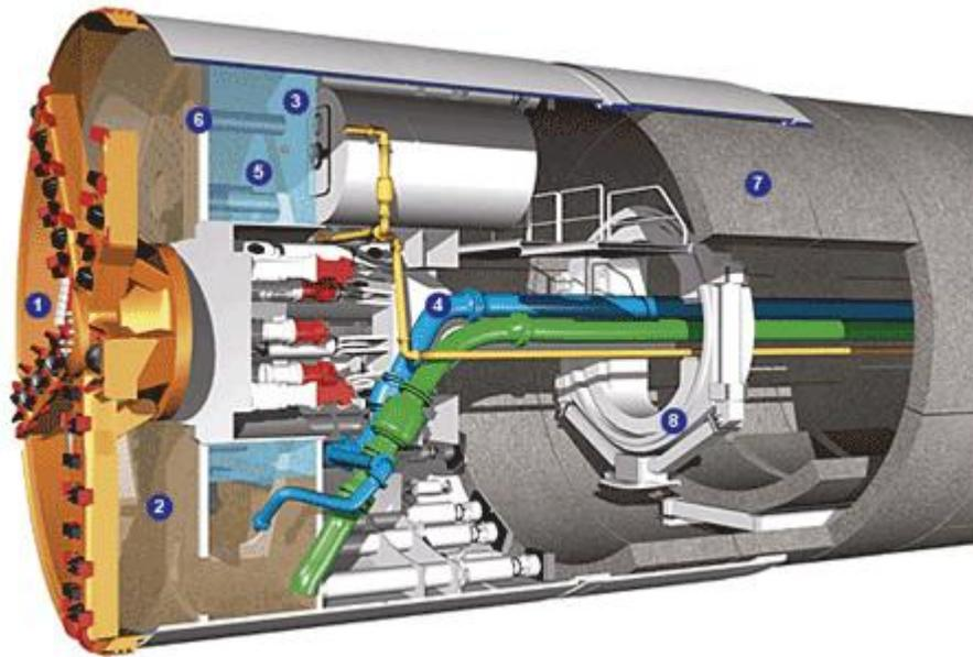
**Diagram 4.3: Schematic of a typical slurry TBM**
