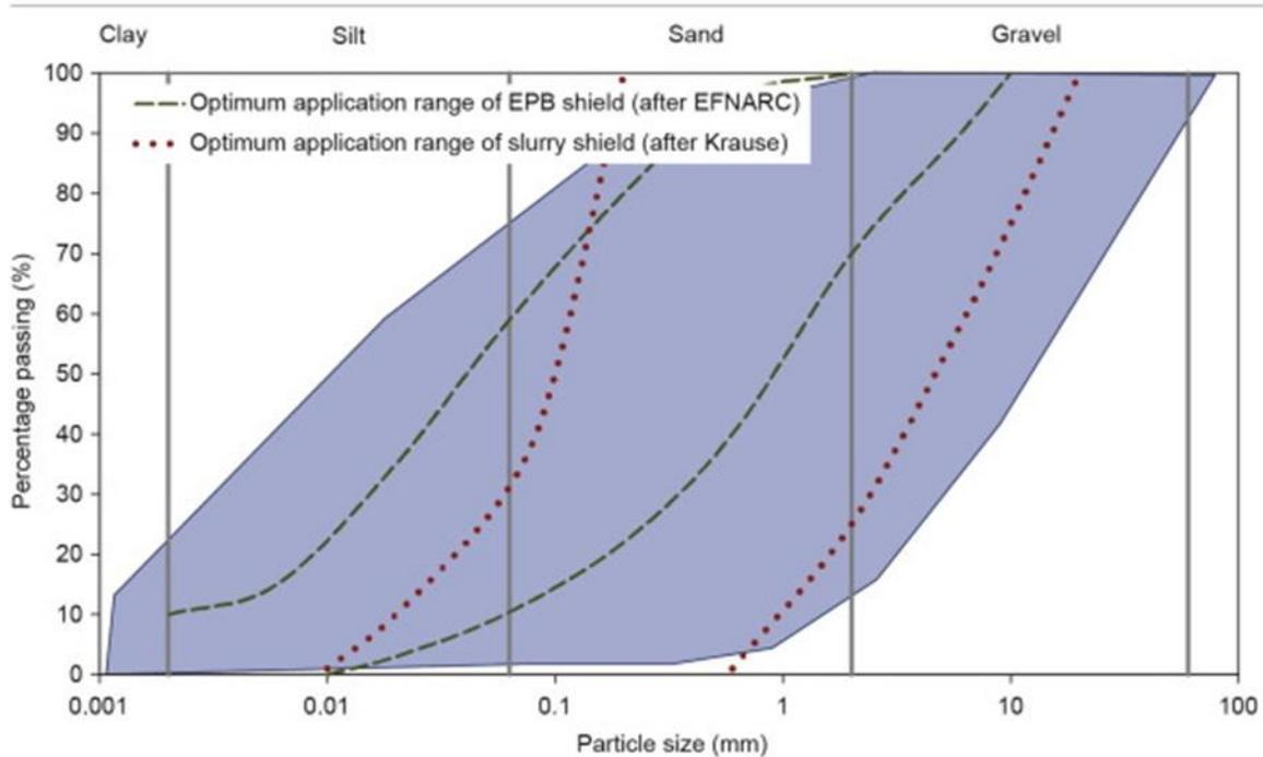
Diagram 4.4: Applicable particle sizes for the TBM types from Mechanised Tunnelling in Soft Soils (Zumsteg and Langmaack, 2017)
