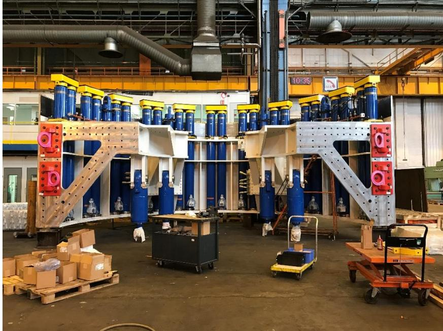
**Diagram 4.13: A section of TBM shield shove rams installed in the factory**
