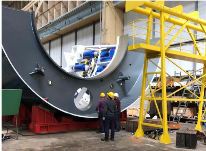
**Diagram 4.11: Bottom half of the front shield of a two-part machine in the factory**
