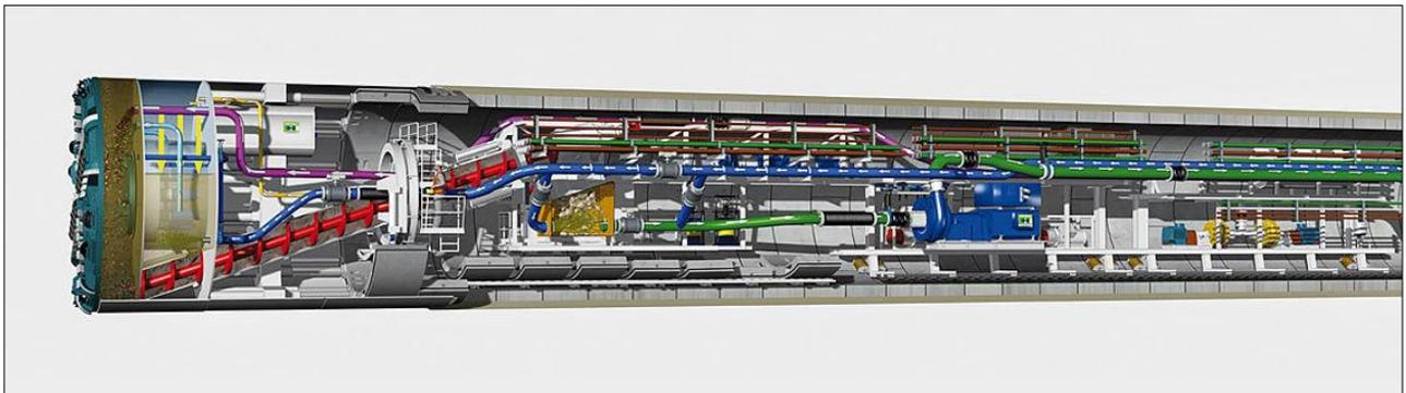
Diagram 4.5: Variable density slurry TBM (from Herrenknecht)
