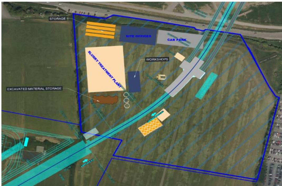
**Diagram 2.4: Dublin Airport South Portal: Indicative Site Layout during TBM Tunnelling**
