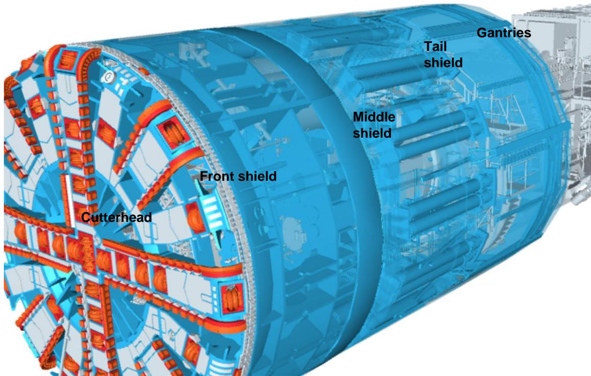
**Diagram 4.9: Cutterhead, front, middle and tail shields of a TBM**
