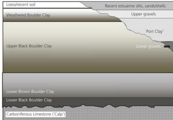
**Diagram 3.2: Simplified schematic of the interpreted stratigraphy of the DBC (Skipper et al., 2005)**
