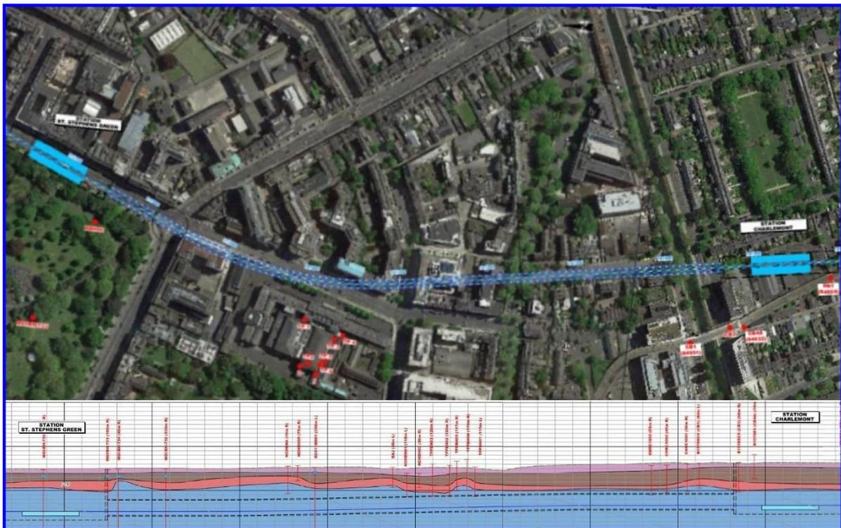
Diagram 3.14: Geologic Profile for TBM Drive C9- St Stephen's Green to Charlemont
