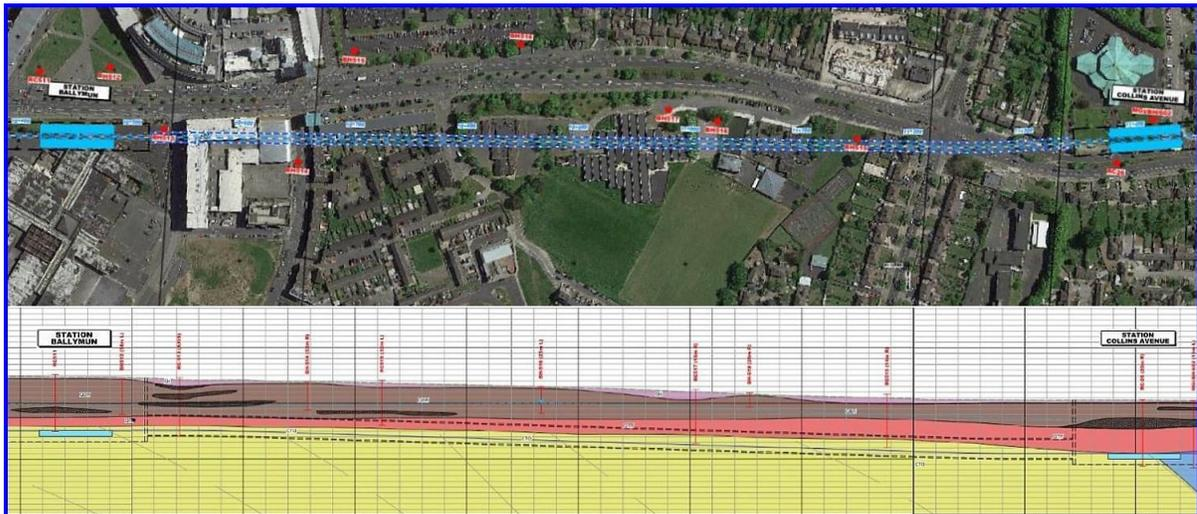
Diagram 3.7: Geologic Profile for TBM Drive C2 Ballymun to Collins Avenue
