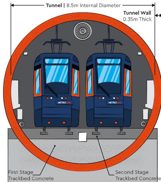
**Diagram 5.1: Bored Tunnel Track Bed Concrete**
