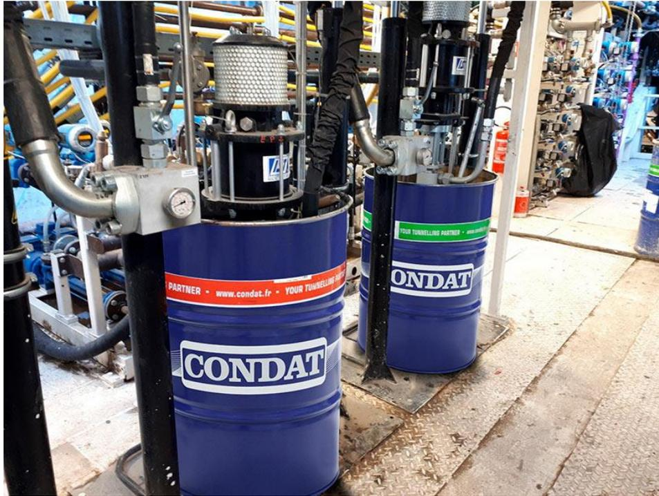
Diagram 2.4: Main Bearing and Labyrinth Grease on a TBM
