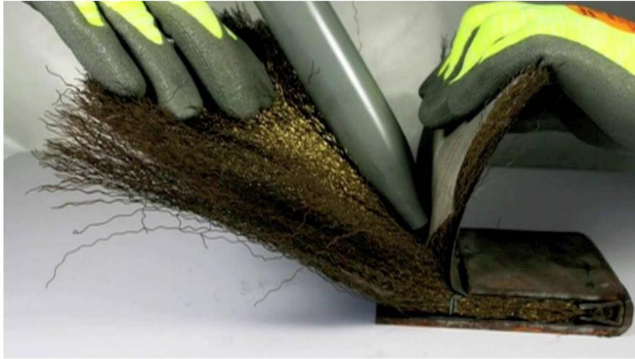
**Diagram 2.7: Single Tail Seal Brush with Hand Packing Injector Tool**
