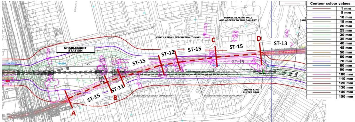
Figure 6-5: Settlement Contours Around Charlemont Station Bridges (ST-11 and ST-12)
