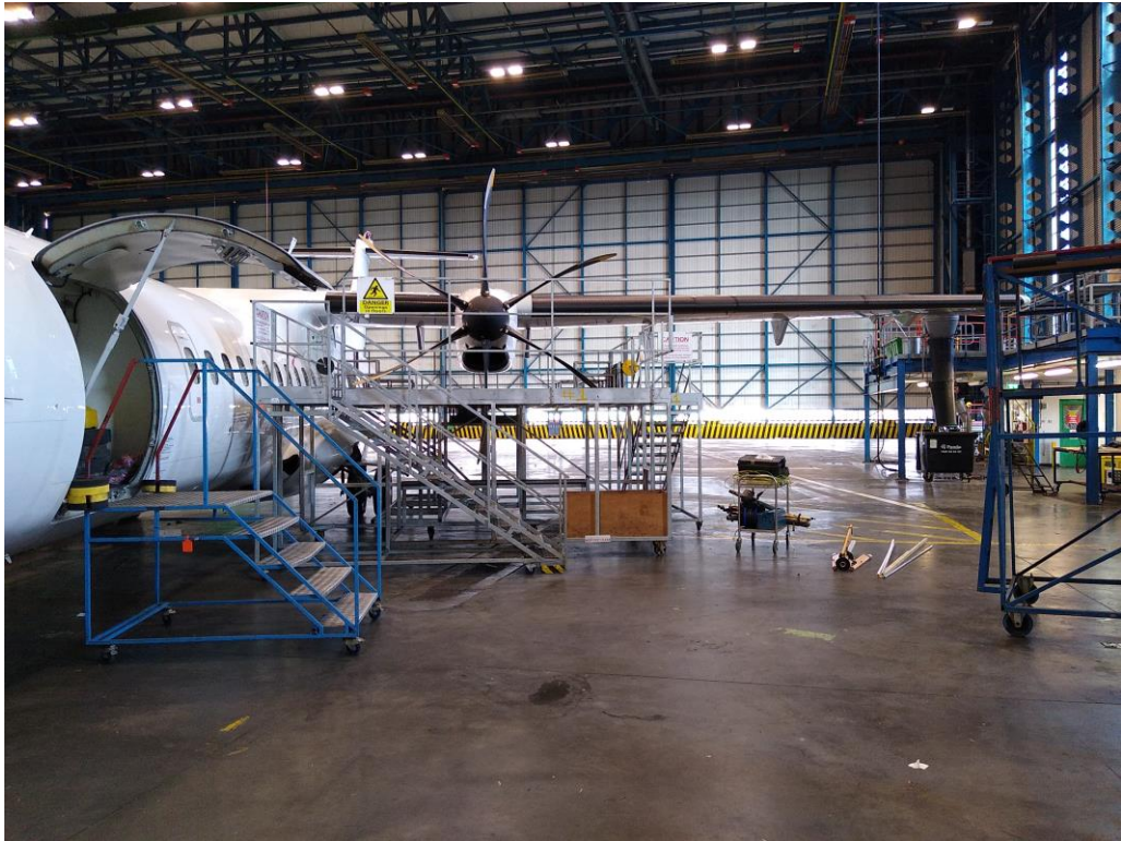
Figure 5: Mobile stairways and gantries surrounding aircraft
