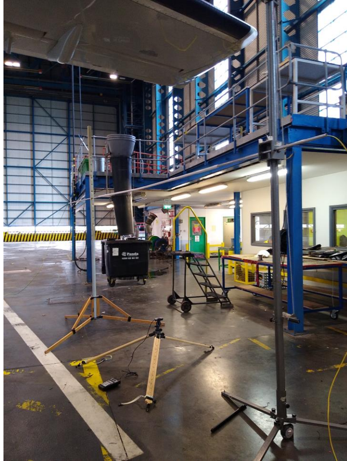
Figure 3: Magnetic Field source installed below wing
