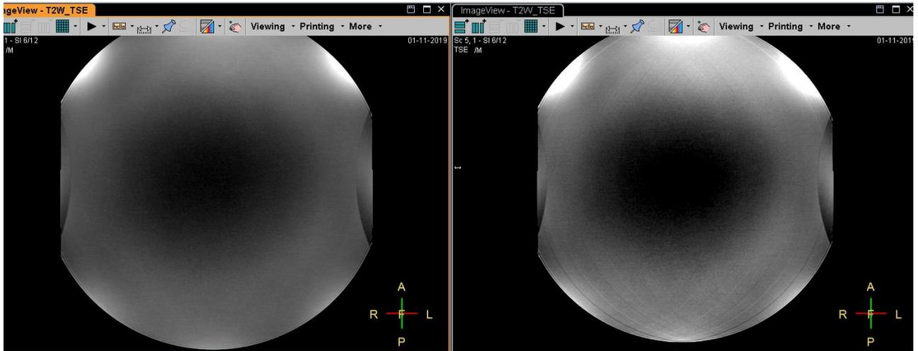
Figure 8: Baseline scan of test artefact (right) versus scan with varying DC field applied
