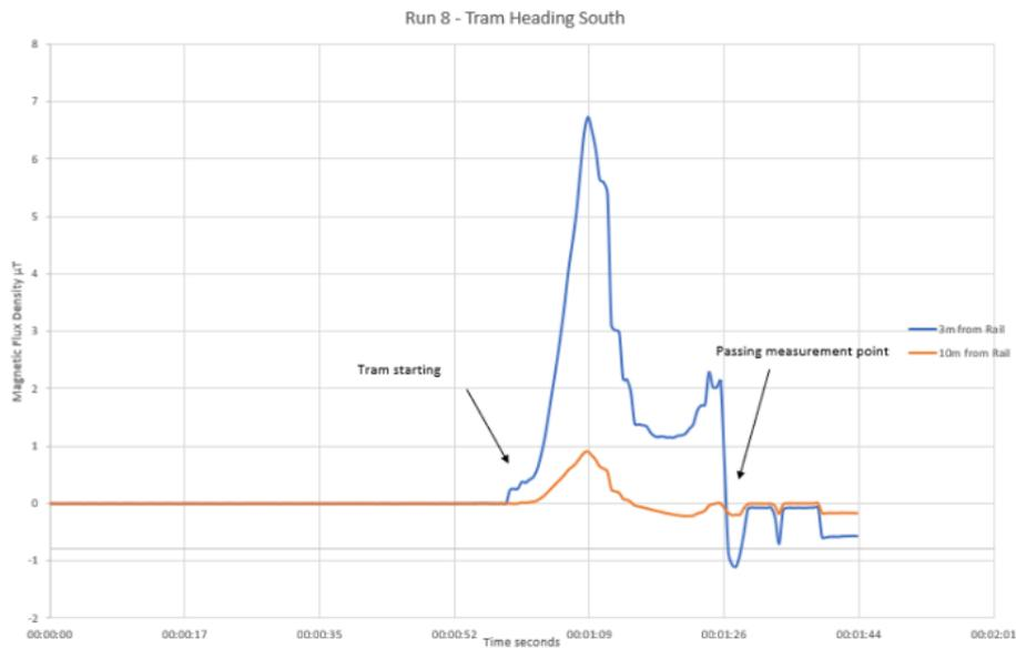
Figure 3: Magnetic flux profile of Luas passing measuring point at 3 m and 10 m distance
