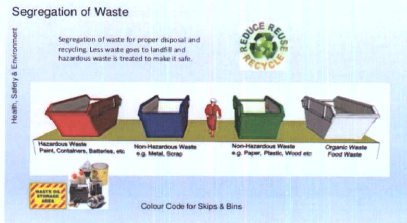
Figure 5.1: Waste segregation skips
