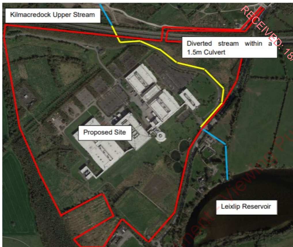
Figure 14.3: Diverted Stream within the KIC Site.
