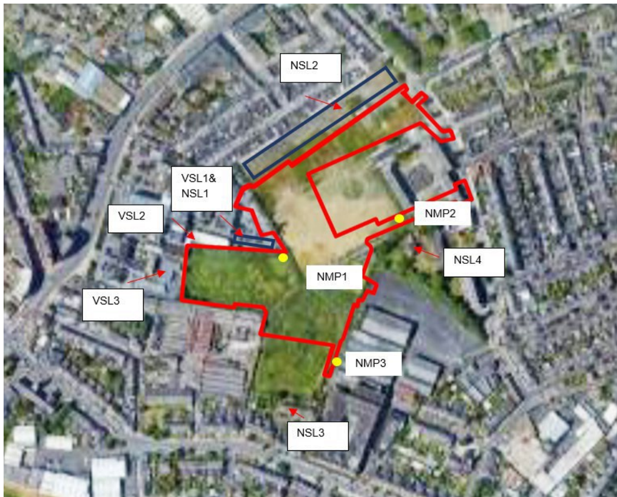
Figure 7-1 Locations of Noise Monitoring Points (NMPs), NSLs and closest VSLs (Blue boxes represent new buildings not shown on aerial photography)
