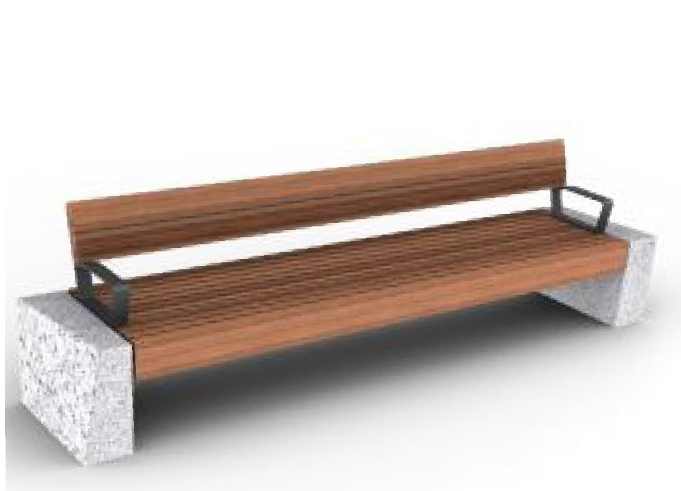
V49S Seat with Backrest / Armrest Supplier: Omos Material: Honed Granite / Hardwood / Hot dipped galvanised mild steel. Powder coated finish. Above Ground Dimensions: 3000mm(l) x 600mm (w) x 831mm (h)
