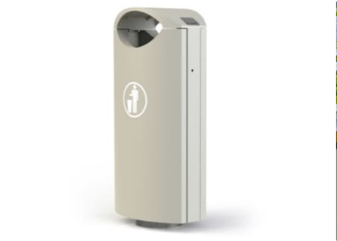
s16.2 Litter Bin Supplier: Omos Material: Hot dipped galvanised mild steel. Cast aluminium hood. All powder coated finish. Colour: Silver decal. Above Grounds Dimensions: 386mm (l) x 1212mm (h) x 550mm (w)
