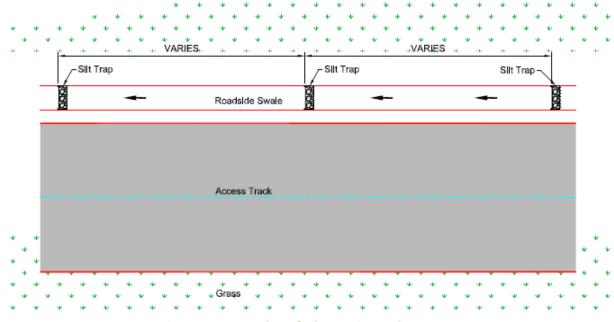
Figure 4-5:Plan of Silt Trap in Swale
