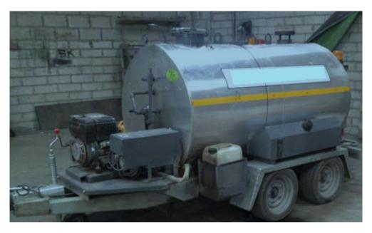
Plate 3-7: Towable Sprayer for Temporary Reinstatement
