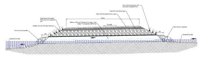
Plate 3-1: Piped Culvert Crossing Long Section
