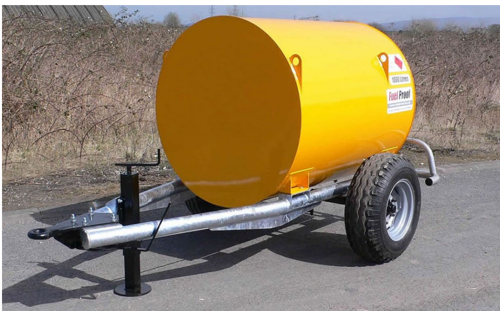
Figure 4-1: Typical Mobile Fuel Bowser
