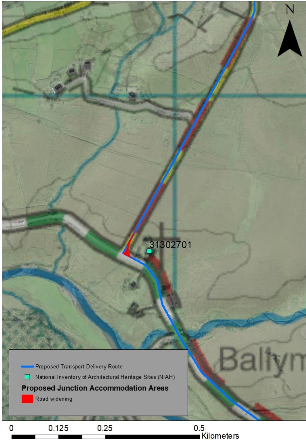
Figure 12-12: Junction accommodation area at Tawnaghmore Td.
