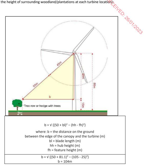
All turbines are positioned outside the recommended 104m buffer zone.
