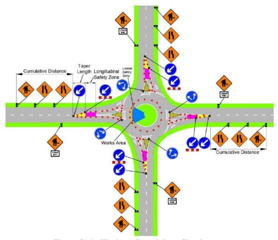
Figure C16 – Works on Roundabout Circulatory
