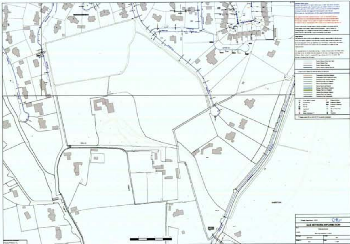
Figure 12.2 – Existing Gas Network Layout
