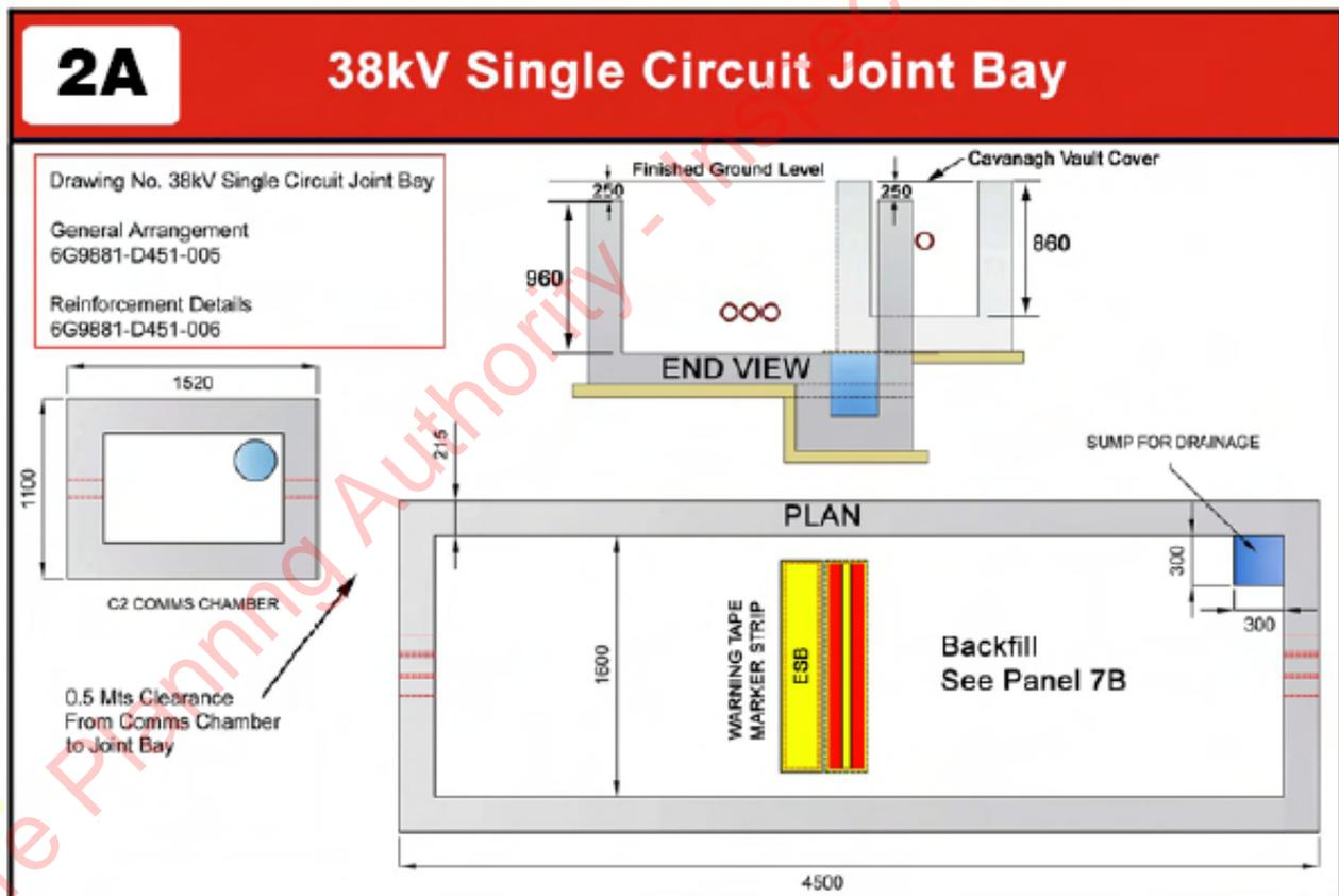
Figure 3-7: ESBN 38kV Single Circuit Joint Bay
