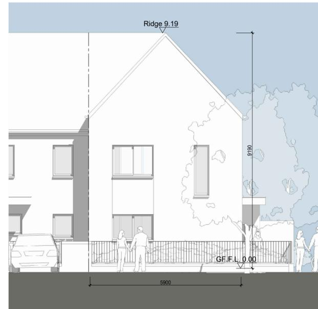
HT C3 - Proposed Front Elevation
