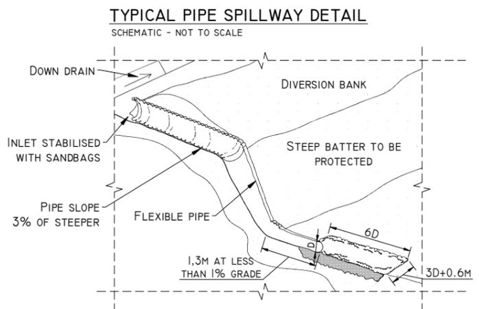
**TYPICAL PIPE SPILLWAY DETAIL**
