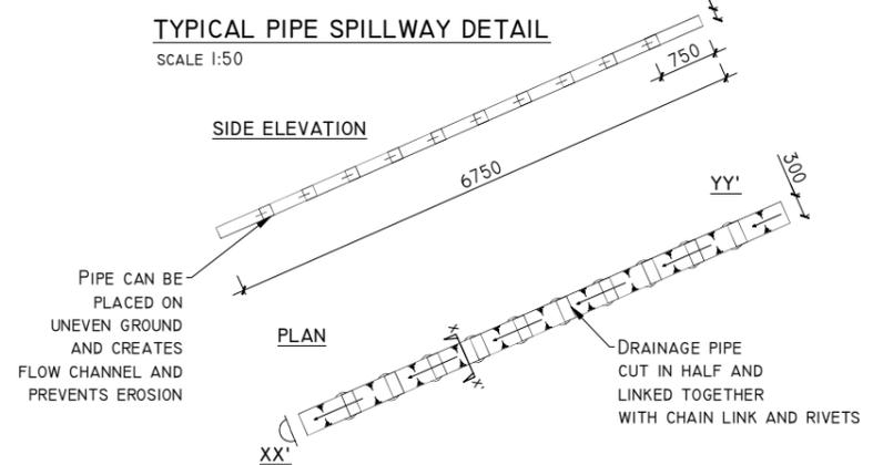
**TYPICAL PIPE SPILLWAY DETAIL**
