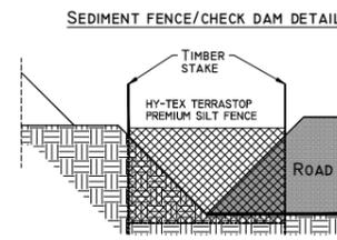
**SEDIMENT FENCE/CHECK DAM DETAIL**
