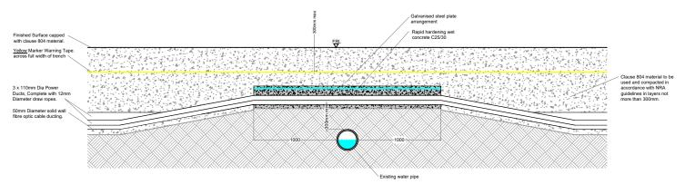
Option C - Flat bed over existing pipe - 33kV SCALE 1:20
