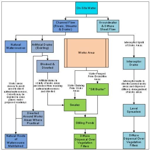
Figure 4-13 Proposed Development Drainage Process Flow
