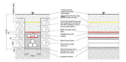
Option A - Cross section - 110kV SCALE 1:20
