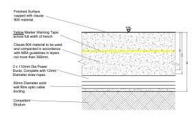
Option A - Cabling Cross Section - 33kV SCALE 1:20
