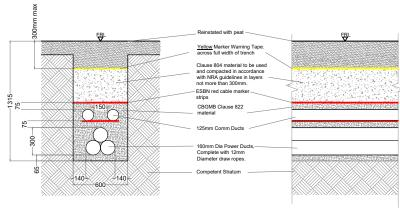
Option A - Cross section - 110kV SCALE 1:20
