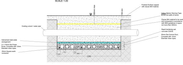
Option B - Flat bed under existing pipe - 33kV
