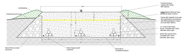
Option A - Cabling Cross Section - 33kV
