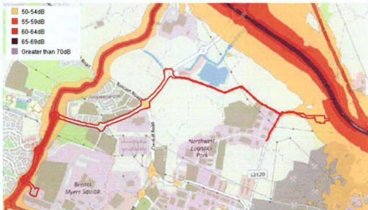
Figure 7.4 L night contours for road traffic noise
