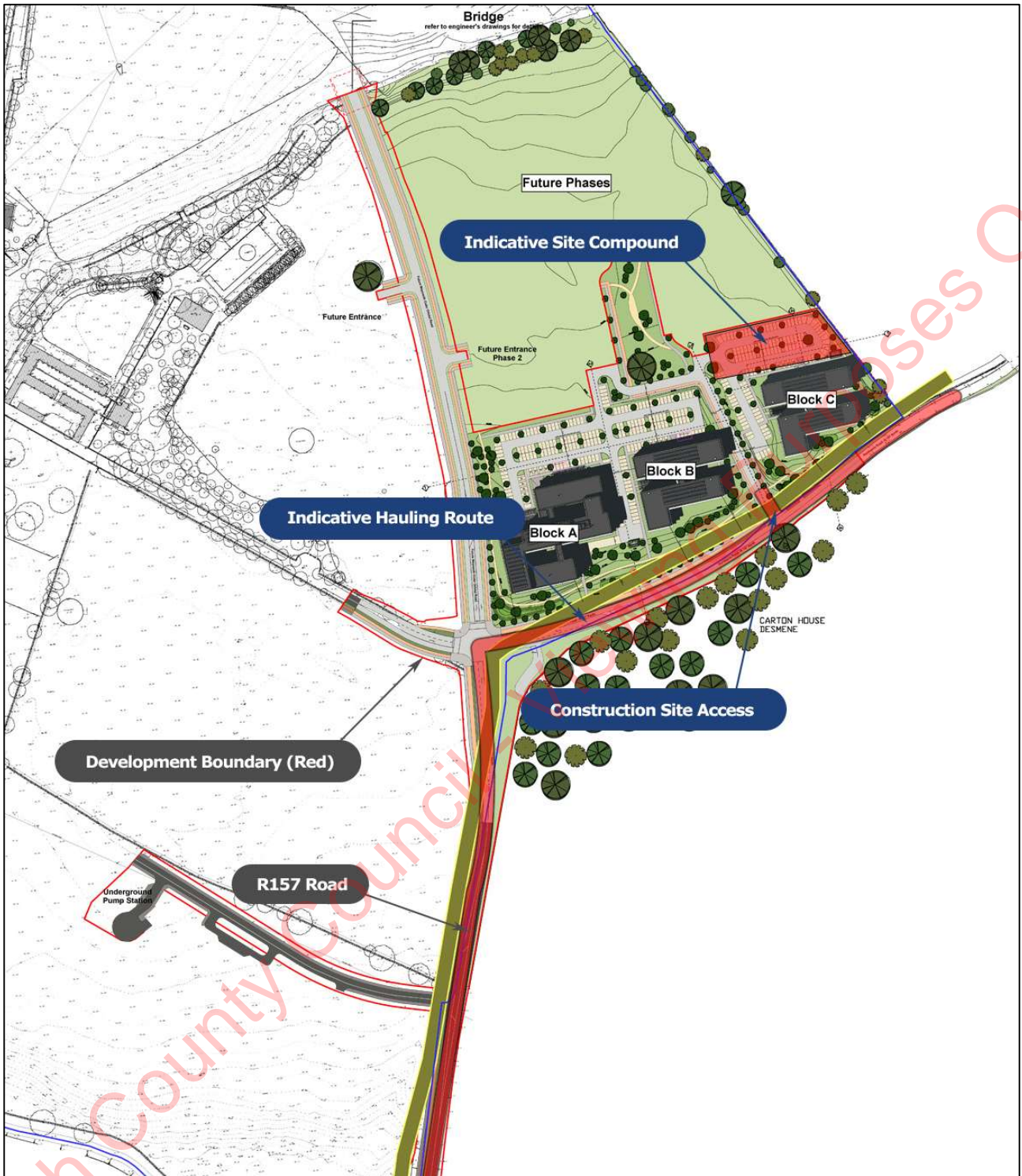
Figure 4: Indicative Site Compound and Hauling Route
