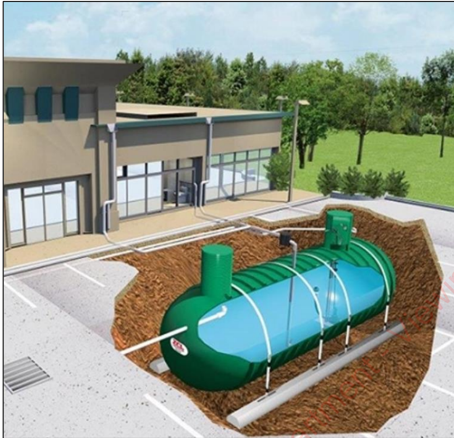
Figure 4-7 Example of Rainwater Harvesting System
