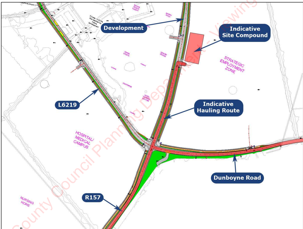
Figure 9: Indicative Site Compound and Hauling Route
