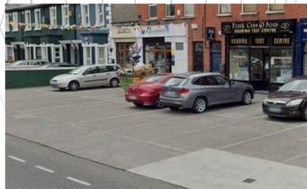
THE CURRENT DISPOSAL OF CAR PARKING BAYS IS A POTENTIAL HAZARD FOR PEDESTRIANS BECAUSE IT HAS TO BE INVADDED IN THE ACCESS TO PARK. THIS AREA IS REMOVED IN THE DESIGN PROJECT AND NEW CAR PARKING DISPOSED IN PARALLEL BAYS.
