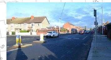
A CONTROLLED CROSSING IS PROPOSED IN THE DESIGN PROJECT WHERE AN UNCONTROLLED CROSSING CURRENTLY EXISTS. A L-SHAPED STEM SHOULD BE PROVIDED AND ACCESSIBILITY MEASURES FOR THIS TYPE OF CROSSING.
