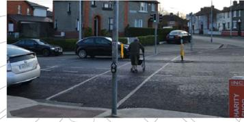
L-SHAPED STEM IN CONTROLLED CROSSING SHOULD BE EXTENDED TO THE BUILDING LINE. IF THE CENTRAL ISLAND IS INTENDED AS AN AREA TO WAIT AS PER TIME OF CROSSING; THEN RED BLISTER TACTILE PAVING SHOULD BE PROVIDED.
