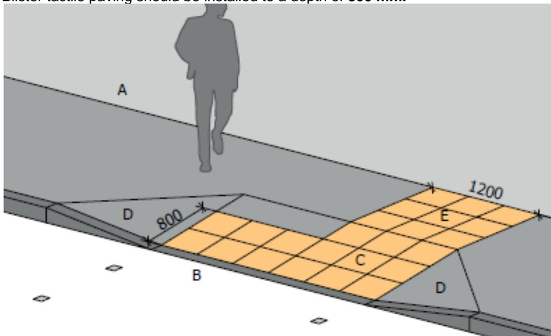
**Figure 11. Uncontrolled Crossing at Side Road**
