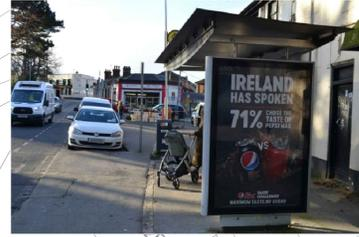
THE LOCATION OF THE SHELTER IN BUS STOP SHOULD BE RECONSIDERED TO ALLOW PEOPLE WITH MOBILITY IMPAIRMENT TO MOVE WITH NO HAZARDS. A MINIMUM DISTANCE OF 1200MM SHOULD BE ENSURED IN ALL SIDES OF ACCESS TO THE BUS STOP THERE IS A CONFLICT WITH THE DRAINAGE CANAL IN THE PICK UP POINT. A KASSEL KERB SHOULD BE PROVIDED WITH AN OPTIMUM RISE HEIGHT OF 180MM TO ADAPT TO LOW-FLOOR BUSES AND THEIR KNEELING SUSPENSION.
