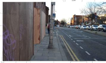
CHECK FOOTPATH WIDTH WHILE OUTDOOR WORKS. A WIDTH OF 1500 MM SHOULD BE ENSURED AND 1200 MM IN A LENGTH OF 2000MM.
