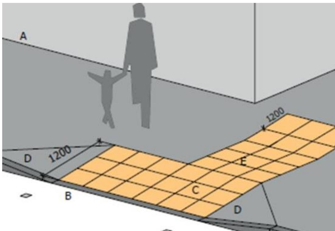
**Figure 9. Uncontrolled Crossing. In line**
