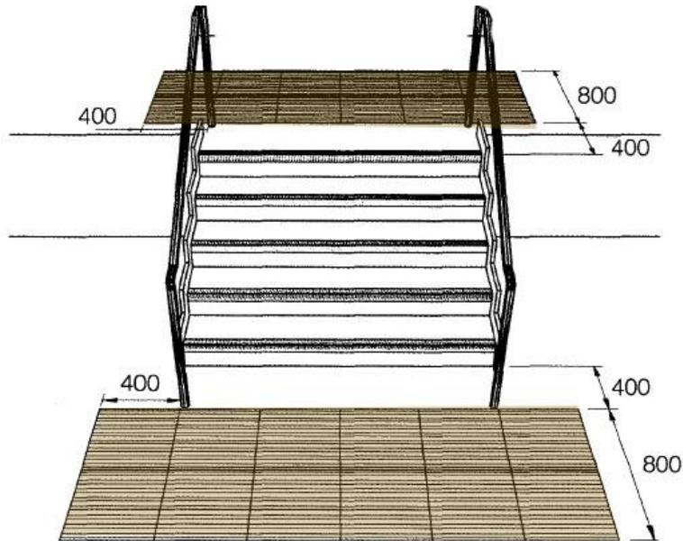
**Layout of corduroy hazard warning surface at the top & bottom of a flight of stairs**
