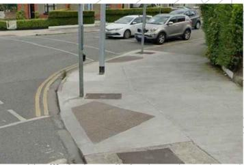
IN CONTROLLED CROSSING POINTS THE L-SHAPED STEM SHOULD EXTEND TO THE REAR OF THE FOOTPATH.
