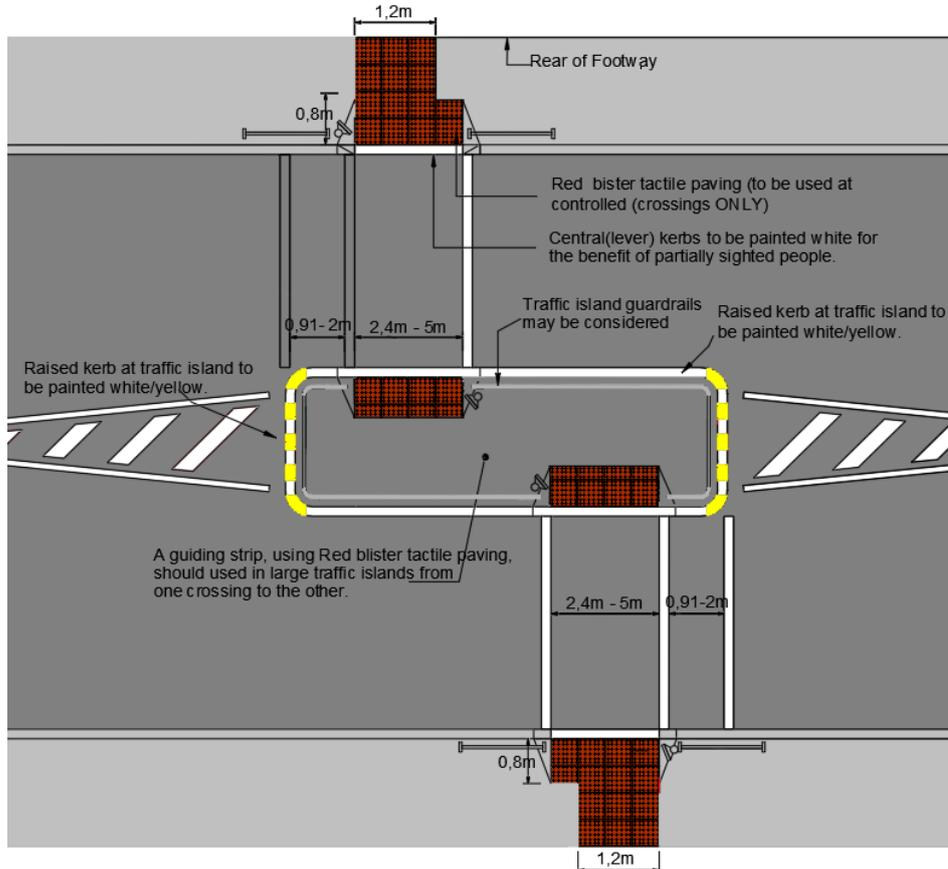
**Figure 18. Controlled Crossing. Staggered Signalized Crossing**
