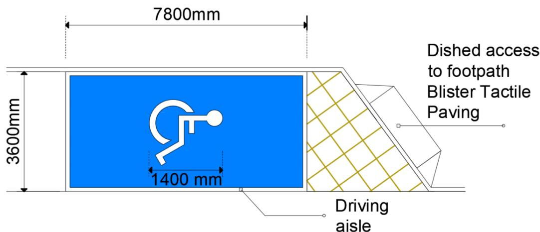
**Figure 3. Example of Parallel parking**
