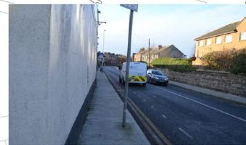
CHECK POSITION OF SIGNAL POLES FOR NOT REDUCING FOOTPATH WIDTH. THE MINIMUM DISTANCES WHEN OBSTACLES CANNOT BE REMOVED SHOULD BE 1500MM. AND 1200 IN SOME POINTS IN A LENGTH OF 2000MM.
