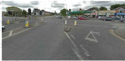
IN THE PROJECT DESIGN THE MULTI STAGE CROSSING WITH UNCONTROLLED CROSSING AND CONTROLLED CROSSING IS REMOVED. THE FOOTPATH BECOMES WIDER IN THE CORNERS AND THE DISTANCE OF CROSSING IS REDUCED. A CONTROLLED CROSSING IS PROPOSED. ACCESSIBILITY MEASURES AS RED BLISTER TACTILE PAVING AND DISHED KERB SHOULD BE IMPLEMENTED, AND AUDIBLE AND SIGNAL DEVICES TO BE INCORPORATED
