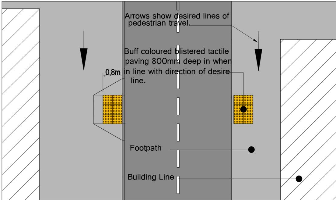
**Figure 12. Uncontrolled Crossing. Not in Direct Line of Travel**
