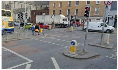
IN THE DESIGN PROJECT THE TRIANGULAR REFUGE ISLAND IS REMOVED AND A DIRECT CROSSING FOR ONLY KEVIN STREET UPPER IS PROPOSED. IF IS NOT ENOUGH THE TIME FOR CROSSING THE CENTRAL ISLAND SHOULD BE CONSIDERED AS AN AREA TO WAIT AND TACTILE PAVING MUST BE INCLUDED.
