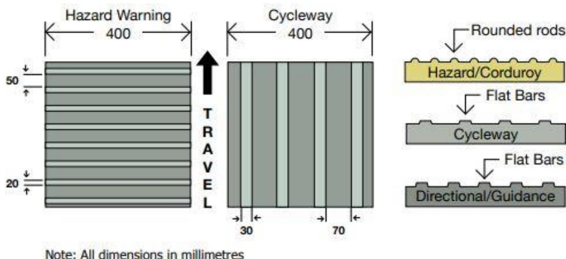
Figure 22. Examples of hazard warning and cycle way paving
