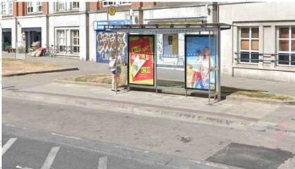
AN ISLAND BUS OPTION IS PROPOSED IN THE DESIGN PROJECT. IT SHOULD BE CONSIDERED FOR AVOID THE PEDESTRIAN/CYCLIST CONFLICT, WITH AN ON-DEMAND SIGNALISED PEDESTRIAN CROSSING (TACTILE PAVING, PUSH BUTTON, LED WARNING STUDS) AND A SECONDARY UNCONTROLLED CROSSING ON THE DOWNSTREAM OF THE ISLAND. DESIGNERS SHOULD NARROW THE CYCLE TRACK TO LESS THAN 2.0 M.
