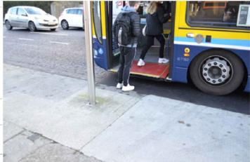
A KASSEL KERB SHOULD BE PROVIDED WITH AN OPTIMUM RISE HEIGHT OF 180MM TO ADAPT TO LOW-FLOOR BUSES AND THEIR KNEELING SUSPENSION.
