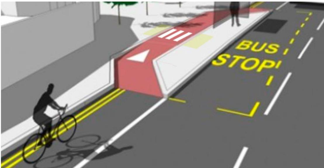
Example of a bus stop bypass solution
