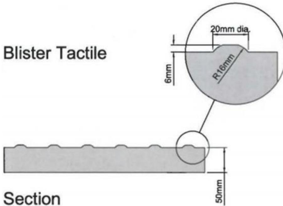
**Figure 19. Blister tactile paving tile and studs dimensions.**
