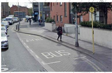
AN ISLAND BUS OPTION IS PROPOSED IN THE DESIGN PROJECT. IT SHOULD BE CONSIDERED FOR AVOID THE PEDESTRIAN/CYCLIST CONFLICT, WITH AN ON-DEMAND SIGNALISED PEDESTRIAN CROSSING (TACTILE PAVING; PUSH BUTTON, LED WARNING STUDS) AND A SECONDARY UNCONTROLLED CROSSING ON THE DOWNSTREAM OF THE ISLAND. DESIGNERS SHOULD NARROW THE CYCLE TRACK TO LESS THAN 2.0 M.
