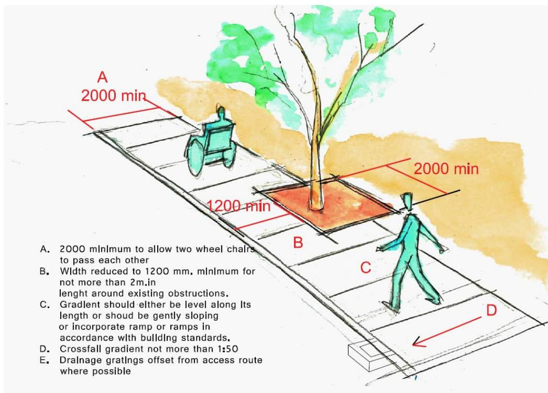
**Figure 5. Urban environment pavement layout**
