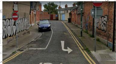
THE WIDTH OF FOOTPATHS IN JUNCTION WITH CLANBRASSIL STREET LOWER SHOULD BE REVIEWED. A MINIMUM WIDTH OF 1500 MM SHOULD BE ENSURED WHEN OBSTACLES CAN NOT BE REMOVED AND 1200 MM. IN A LENGTH OF 2000MM.
