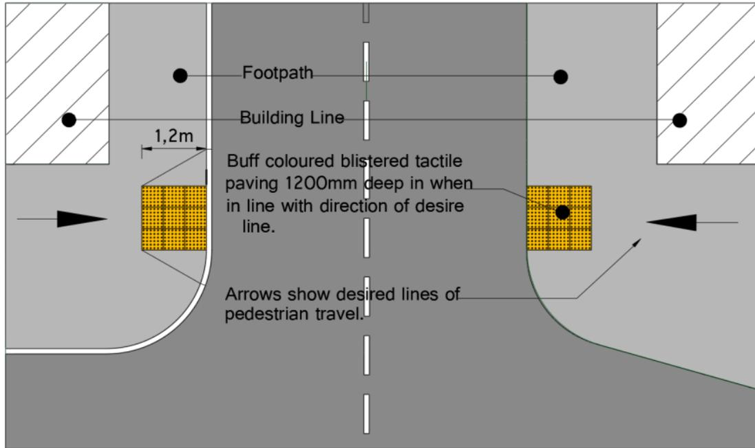
**Figure 10. Uncontrolled Crossing. Direct Line of travel**
