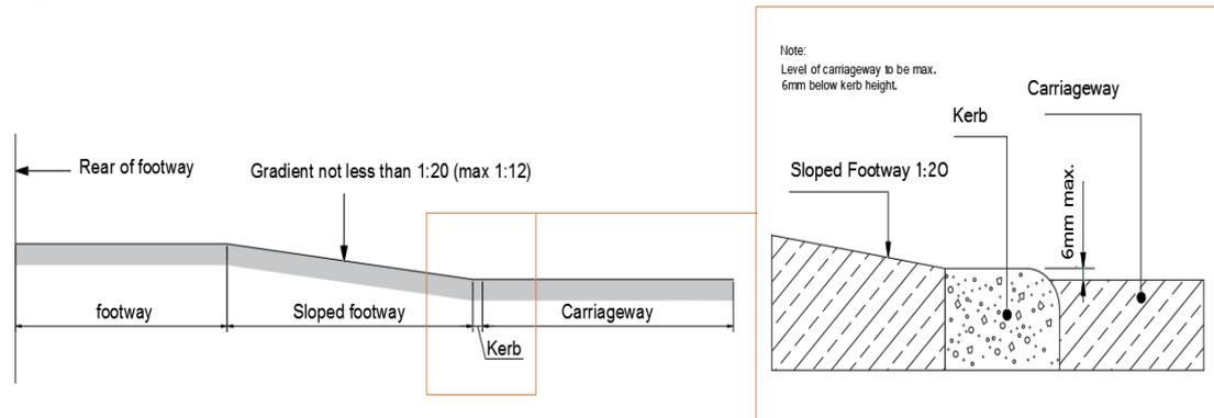
Figure 8. Dished Kerb Section Detail
