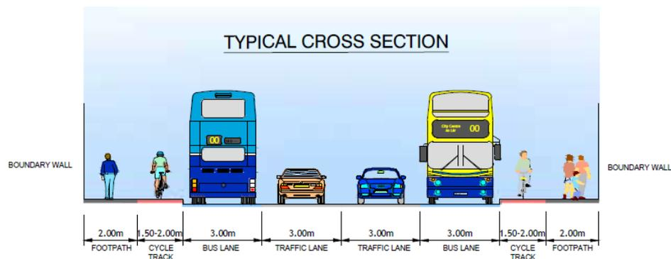
**Figure 6-15 - Typical Cross Section with Cycle Route Option B at Clanbrassil Street Upper**
