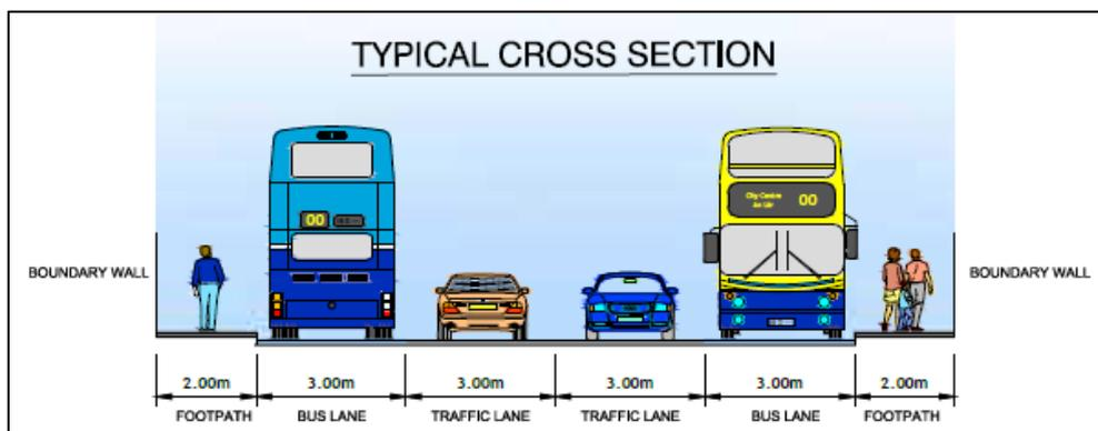
Figure 6-13b– Typical Cross Section for EPR at Clanbrassil Street Upper
