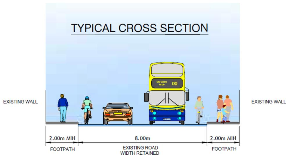
Figure 6-6 - Typical Cross-Section on Kimmage Road Lower in Section 1
