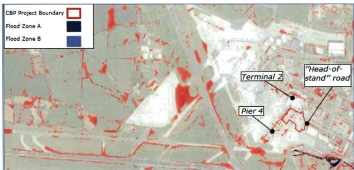
Figure 3-3: Combined Pluvial flood (orange gradient) and Fluvial flood (blue gradient) mapping within Dublin Airport LAP
