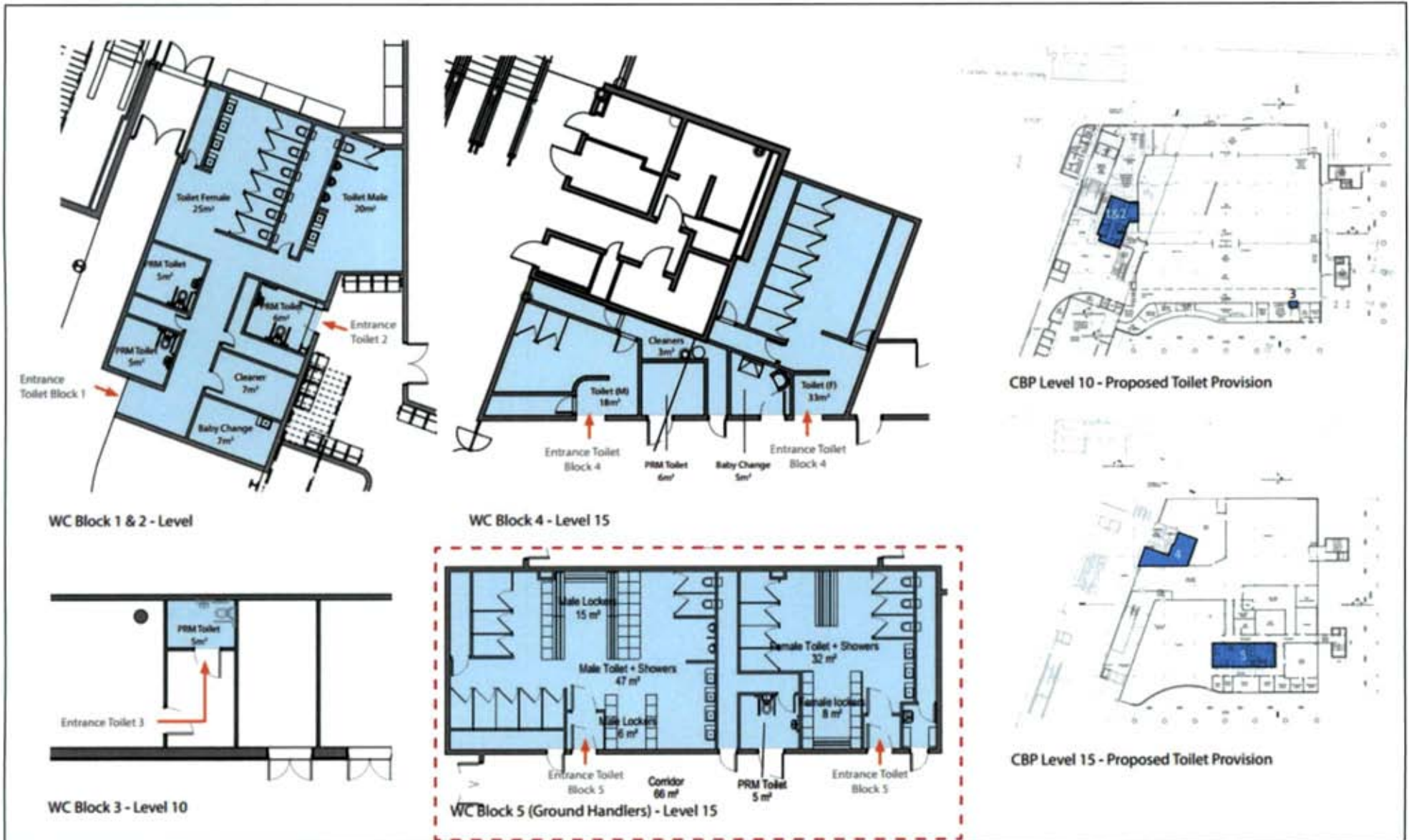
Figure 3-5 - Toilet Block Design (V1)
