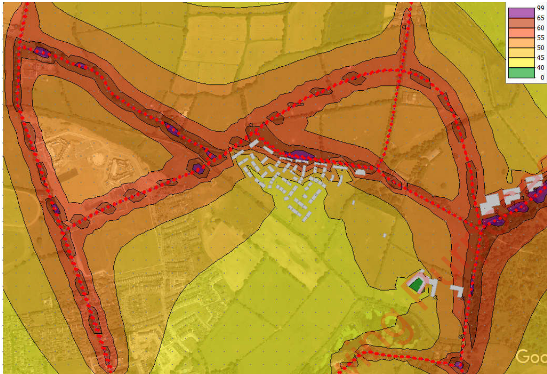
Figure 10-21 Design year 2039 LAeq 16 h levels at 4 m
