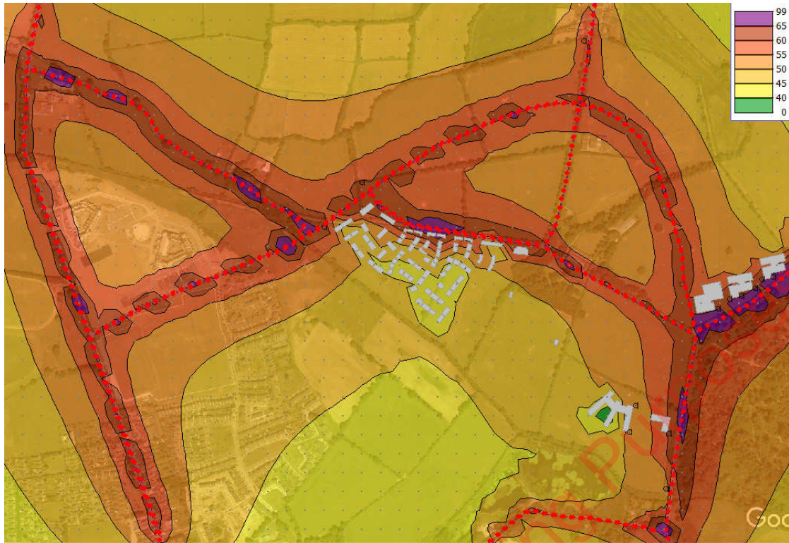
Figure 10-23 Design year 2039 Lden levels at 4 m
