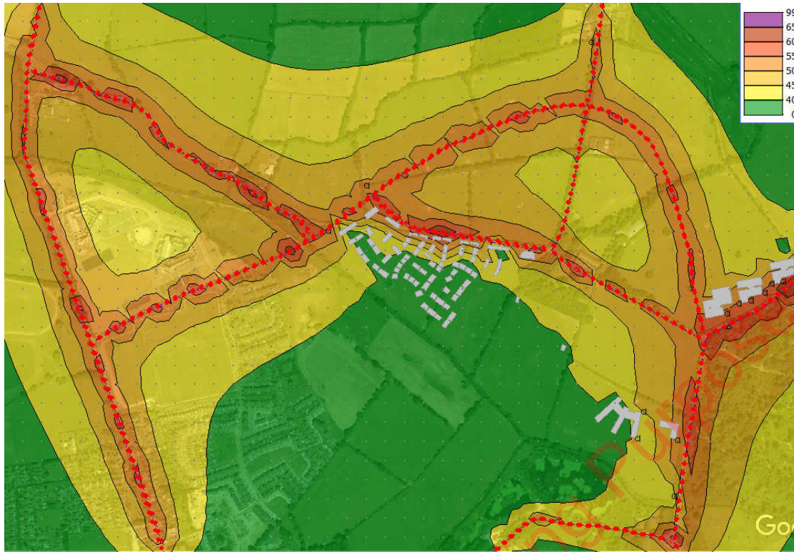
Figure 10-25 Design year 2039 night-time LAeq 1 h levels at 4 m
