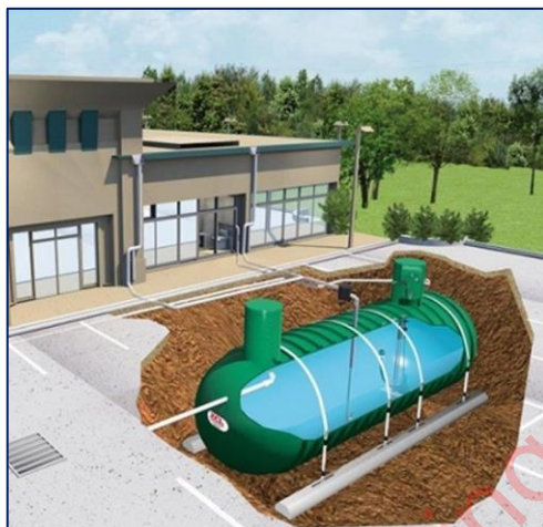
Figure 3.4 - Example of Rainwater Harvesting System
