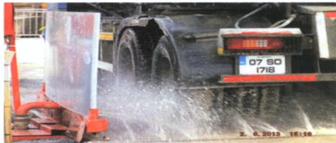
Figure 9 – Typical Wheel Washing Facility
