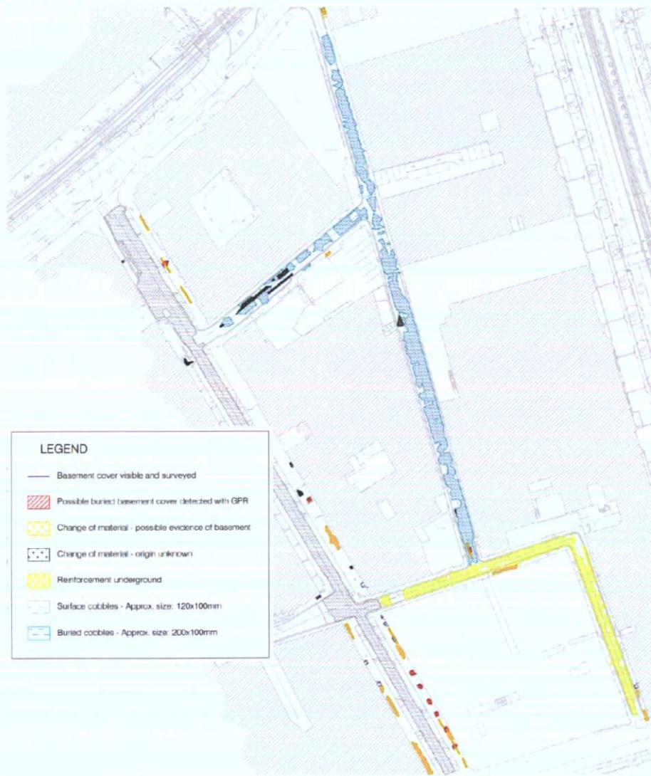
Fig 13: The GPR survey of the internal street network, indicating concealed setts and kerbs, the extent of prior disturbance of which is unknown (Murphy Geospatial)
